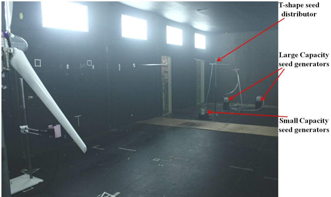
Figure 3-11: Seed generators within the test set-up
