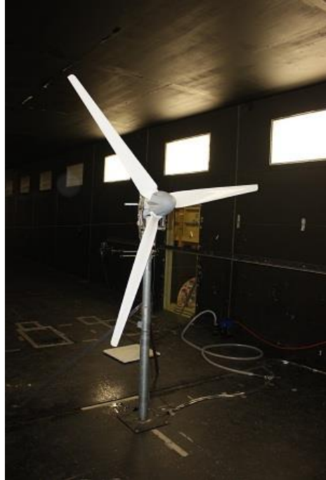
Figure 3-2: Configuration of the upwind three bladed small HAWT rotor in the test set-up
