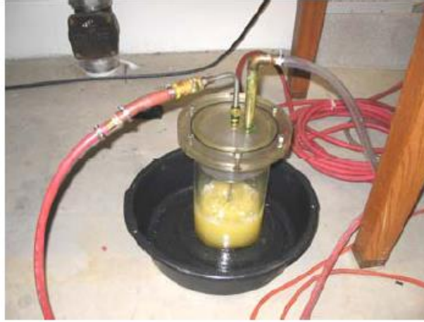
Figure 3-8: Configuration of Laskin nozzle-type particle generator
