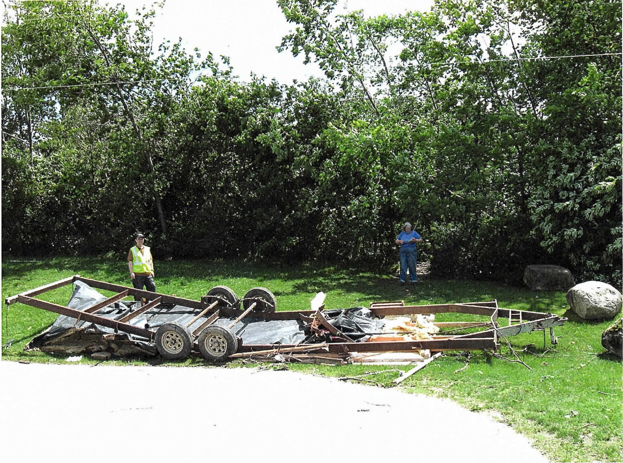
Figure 8: Smith Trailer Park located in Midland. Picture looking southward showing a 42ft trailer frame that had been uplifted and relocated to Erin Rd. where the permanent modular homes were located. The point of origin for this mobile home was measured to be a minimum of 100m from this location.
