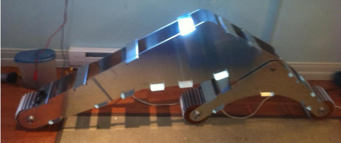
**Figure 4.9: Half Rocker-Bogie Image**
