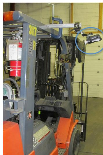
*Figure 4 – Camera on lateral side of the forklift*
