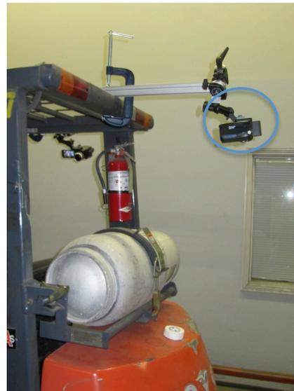
*Figure 6 - Camera at the back of the forklift.*
