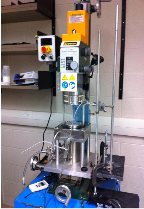
Figure 5-3:UV Irradiance Measurements' setup
