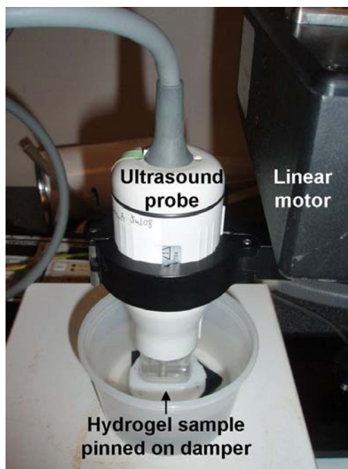
Figure 3.6: Set-up for 3D ultrasound imaging of the hydrogel samples after crossing-paths wear testing. The linear motor translated the ultrasound probe to acquire successive B-mode image planes for 3D images.
