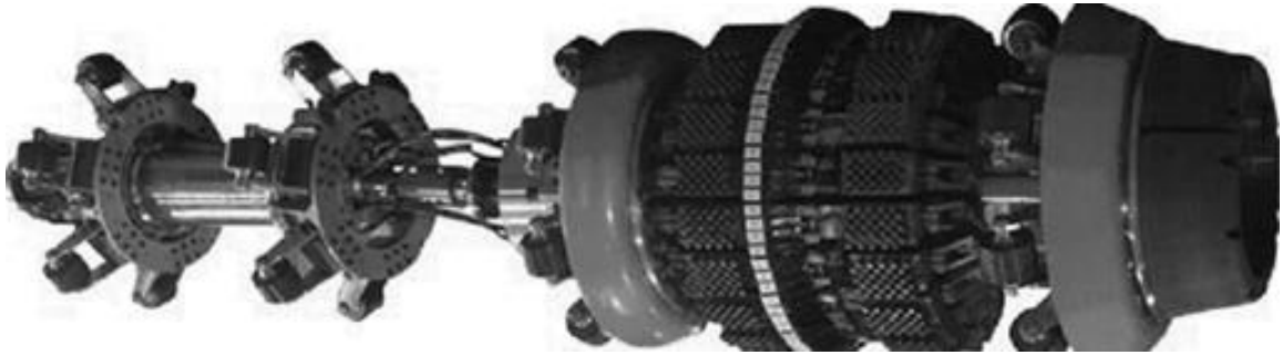
Figure 1.4 A typical in-line inspection tool
