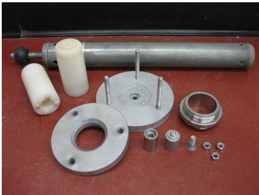
(a) Disassembled compaction cell and standard Proctor hammer
