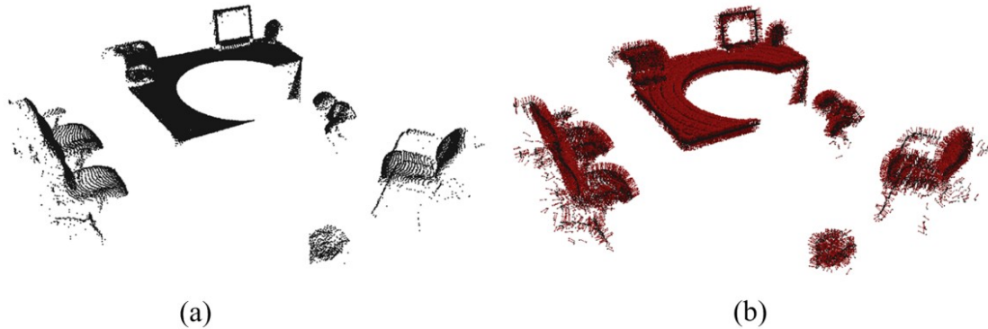
Figure 5.17: (a) Interior point cloud data and (b) Interior points along with their approximated surface normal.
