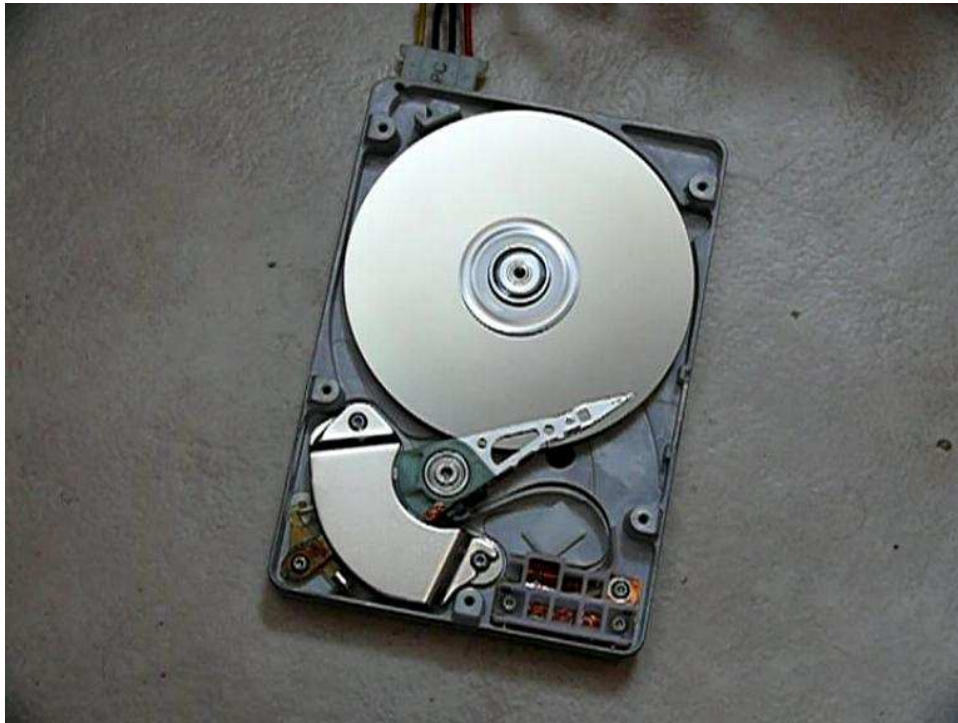
Figure 1.1: The inside of a hard disk drive. It is a device for storing and retrieving digital information. It consists of one or more rapidly rotating discs (storage medium) which is coated with the magnetic layer, read and write heads. This picture is reproduced from [20] under the terms of GNU Free Documentation License.
