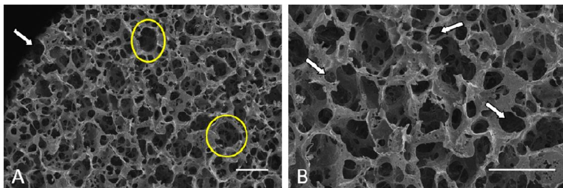
**Figure 4.3: Scanning electron micrographs of porous PCU scaffolds.** Scanning electron micrographs of scaffolds fabricated from PCU with porogens ranging from 180-212 $\mu\text{m}$  in diameter; A) Arrow indicates scaffold edge, pores are highlighted in yellow; B) Arrows indicate interconnecting pores. Scale bar, 250 $\mu\text{m}$ .
