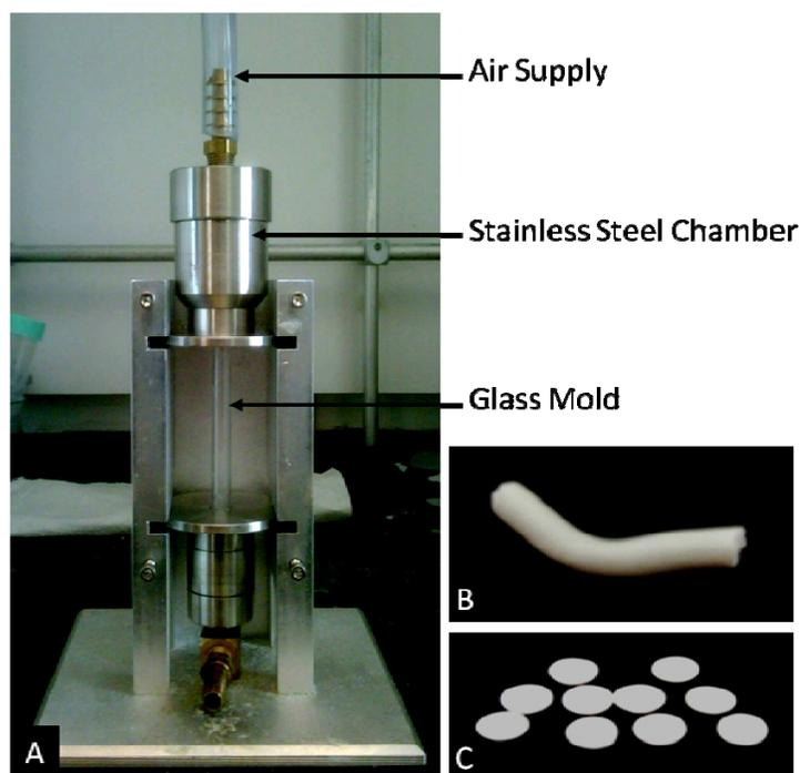
**Figure 3. 1: Scaffold fabrication apparatus.** Apparatus used for fabricating PCU scaffolds using SCLP technique (A); Resulting scaffold after porogen leaching and drying (B); Scaffold discs used for cell culture (C).
