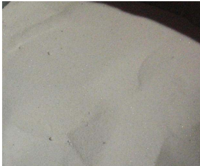
Figure 0II.3: a sample of bed collected sand after spray with “high ALR” nozzle
