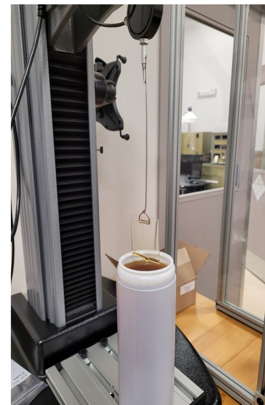
Figure 2: Testing Apparatus of non textured sample in oil
