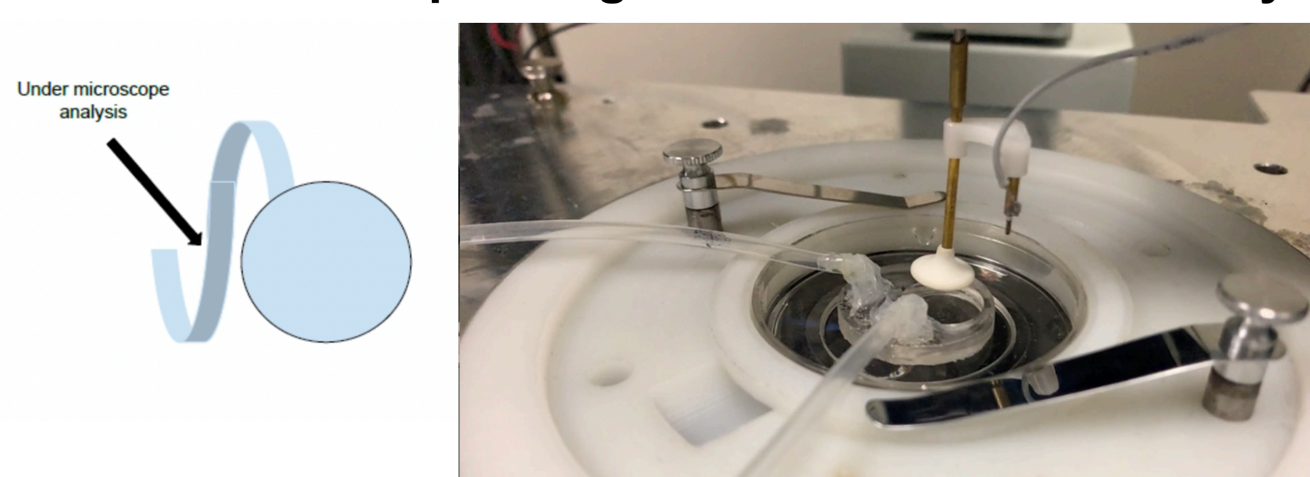
Fig. 1: a) Microfluidic flow channel consisting of a cylindrical reservoir preceding a rectangular channel (nominally 0.5 mm x 0.3 mm).
