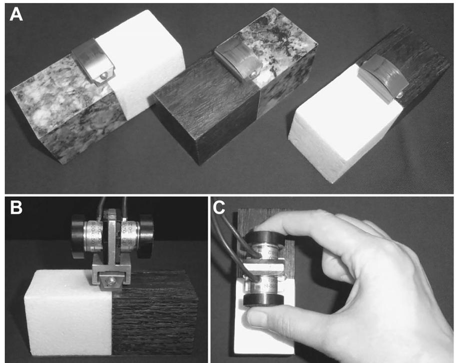
Fig. 1. Stimuli used in *experiment 1*. **A:** the 3 bipartite objects, with halves that appeared to be made of different materials: granite, Styrofoam, and wood. **B:** two 6-axis force-torque transducers were attached centrally to the objects on a small handle. **C:** an object grasped with a precision grip as in the experiment.
