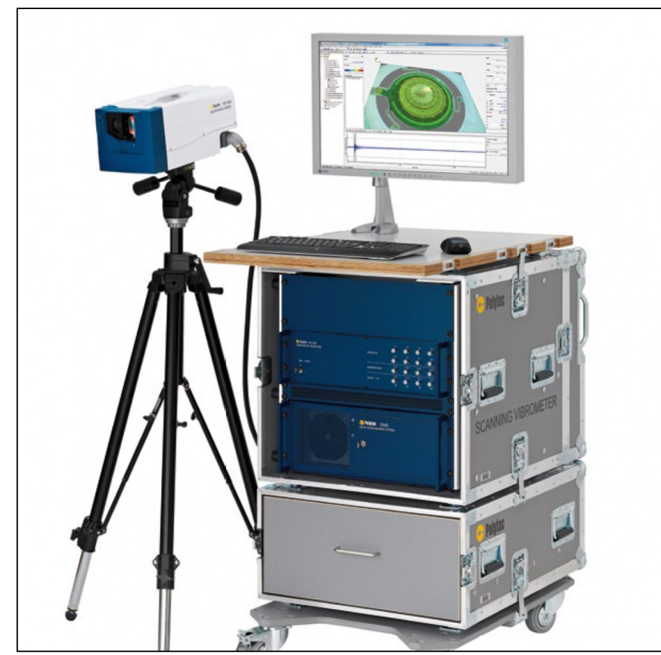
Figure 1 The LDV is used for rapid non-contact measurements of vibrations ($500,000) [1].
