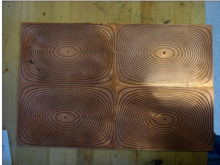
Figure 2.3: The individual quadrants of the y-primary coil prior to being rolled and fastened to the formers.
