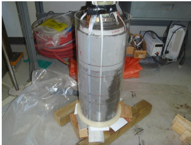
Figure 4.10: A photograph of the basic potting procedure for each layer. A mould was constructed from a plastic cylinder and masking tape and the epoxy was simply poured in and left to set.
