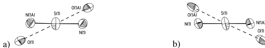
Figure 4.6: View of the dicationic sulfur centre in (a) 4.3NMe 2 and (b) 4.3Ph , interplanar O-S-O and N-S-N angles: 4.3Ph : 25.5° and 4.3NMe 2 : 26.4°.
