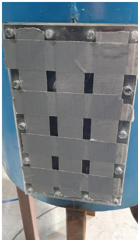
Figure 25 - Secured window of the vessel.
