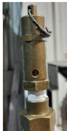
Figure 22 - 10 psi (6.89 kPa) pressure relief valve is included as a safety tool. It's top part moves up to let the extra air leave the vessel.
