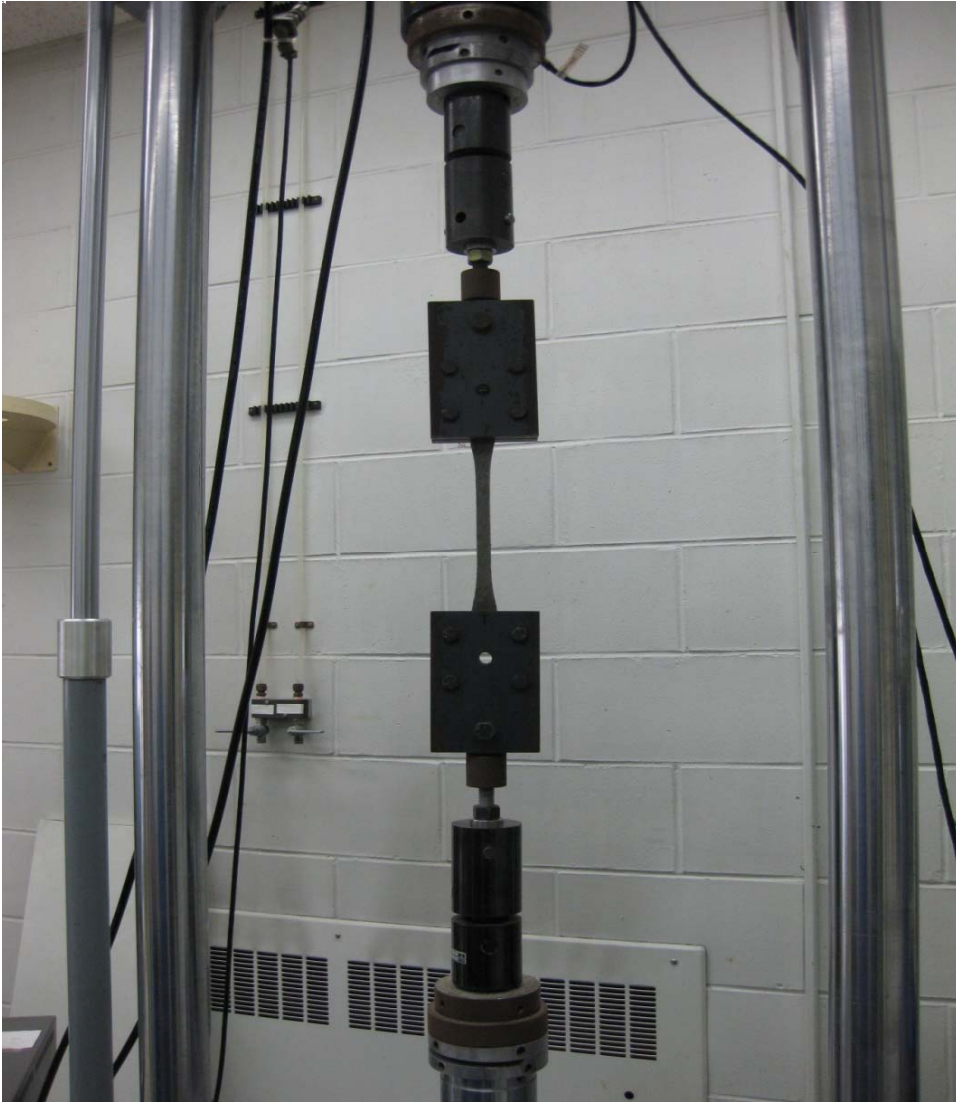
Figure 5.2 Tensile strength test setup
