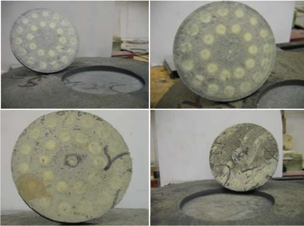
Figure 5.10 Pulled plate surfaces on Sika grout: a) SG-1, b) SG-2, c) SG-3, and d) SG-4
