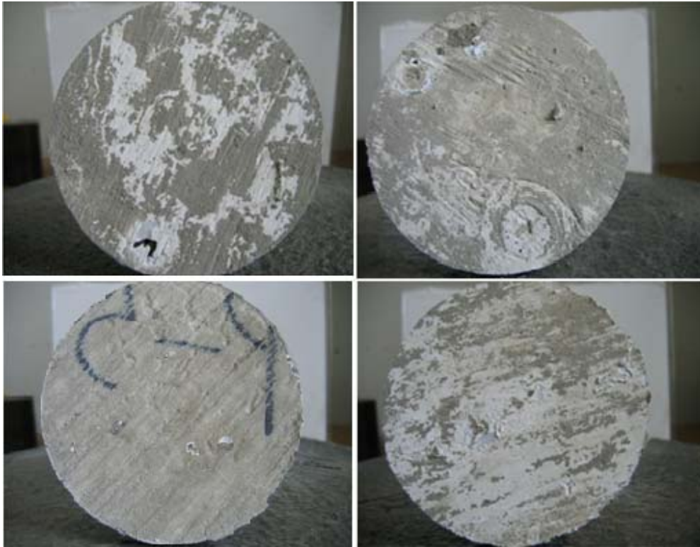
Figure 5.12 Pulled plate surfaces for painted concrete: a) PC-1, b) PC-2, c) PC-3 and d) PC-4
