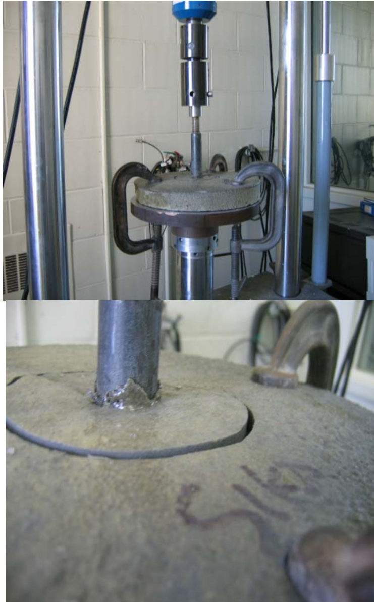
Figure 5.5 The adhesion strength testing setup and pull plate being pulled
