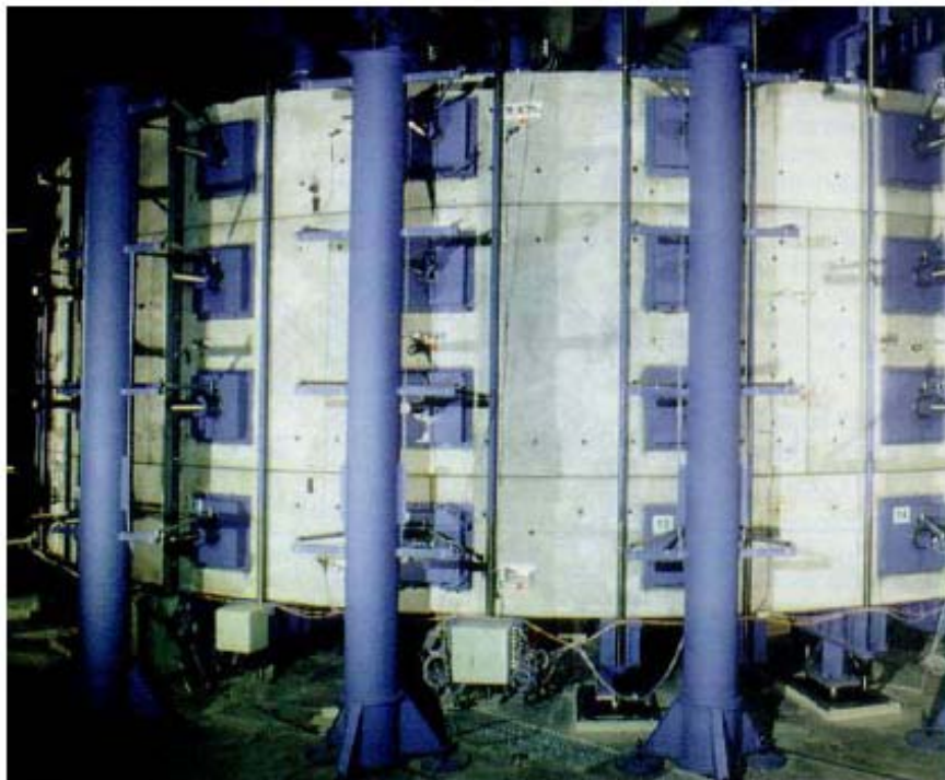
Figure 2.8 The 4 th Elbe highway tunnel lining test (Schreyer and Winselmann, 2000)
