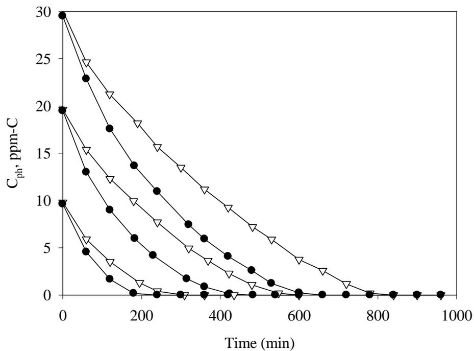
**Figure 50** Influence of 5 ppm of ferric ions on the rate of photooxidation of phenol at different initial concentrations. ( $\nabla$ ) DP P25 ( $\bullet$ ) DP 25 and 5 ppm  $\text{Fe}^{3+}$  in solution
