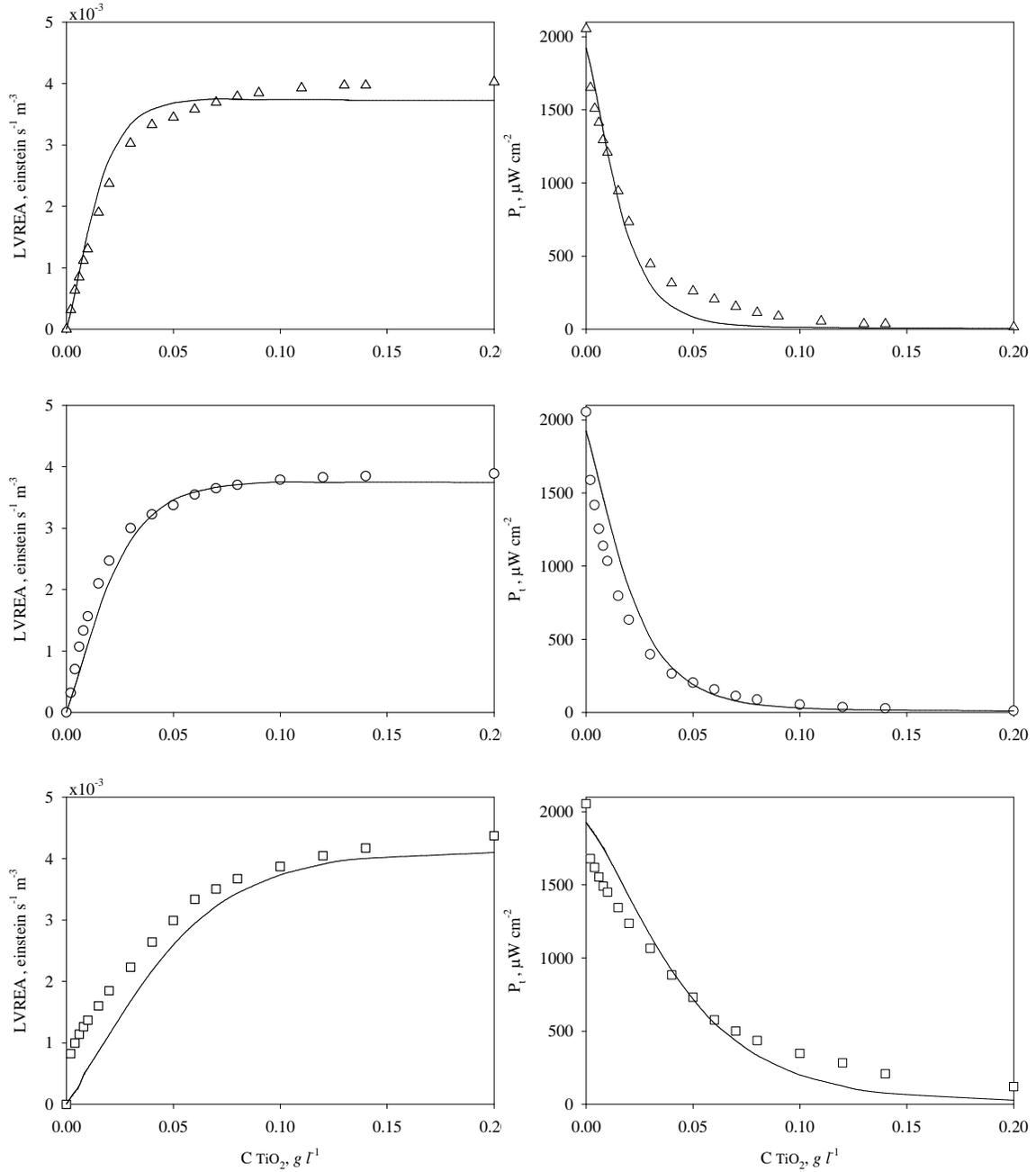
**Figure 26** Experimental results for the LVREA and the transmitted radiation and comparison with “MC simulation 1”. Experimental data: ( $\Delta$ ) DP 25, ( $\circ$ ) Anatase, and ( $\square$ ) Hombikat UV-100 and (—) MC simulations
