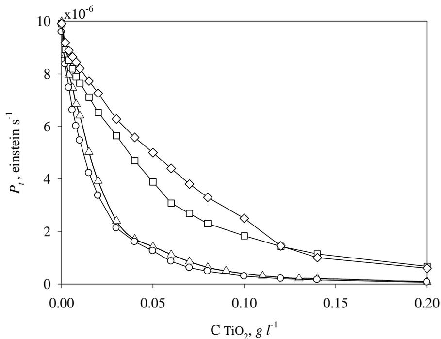
**Figure 19**  $P_t$  vs. catalyst concentration expressed in einstein  $s^{-1}$  when aluminum collimator is used. ( $\Delta$ ) DP 25, ( $\circ$ ) Anatase, ( $\square$ ) Hombikat UV-100 and ( $\diamond$ ) Sol-Gel Cat
