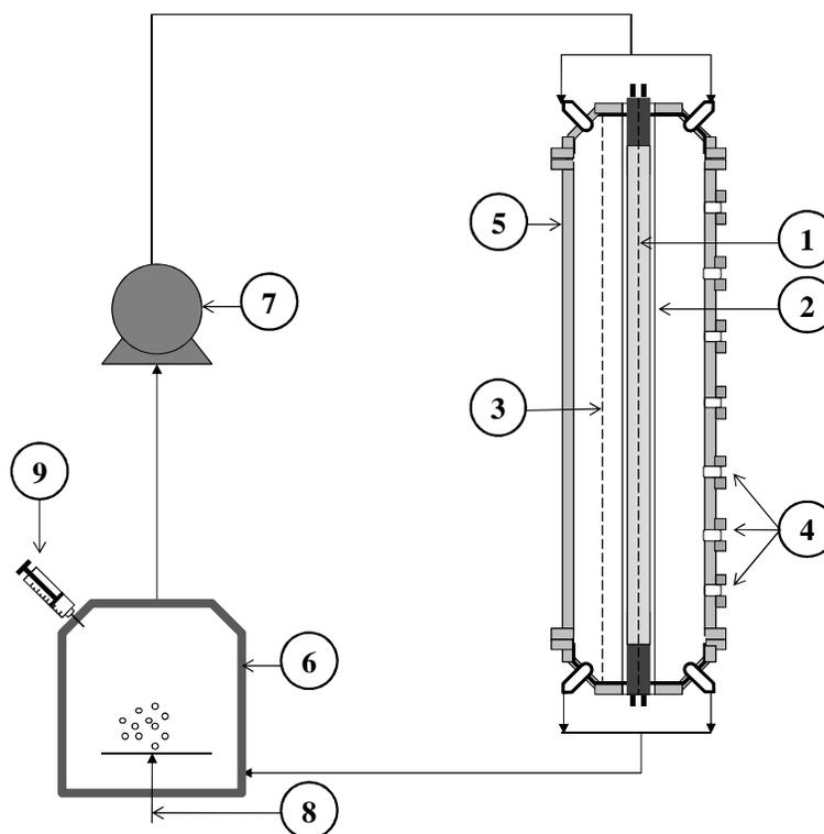
**Figure 7** Schematic representation of the Photo-CREC Water-II reactor
