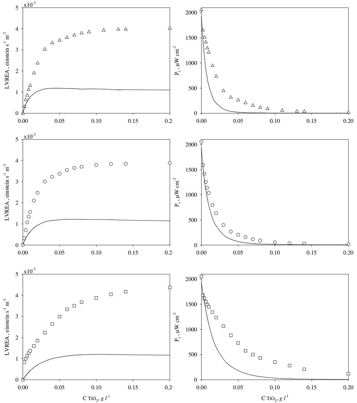
**Figure 27** Experimental results for the LVREA and the transmitted radiation and comparison with “MC simulation 2”. Experimental data: ( $\Delta$ ) DP 25, ( $\circ$ ) Anatase, and ( $\square$ ) Hombikat UV-100 and (—) MC simulations
