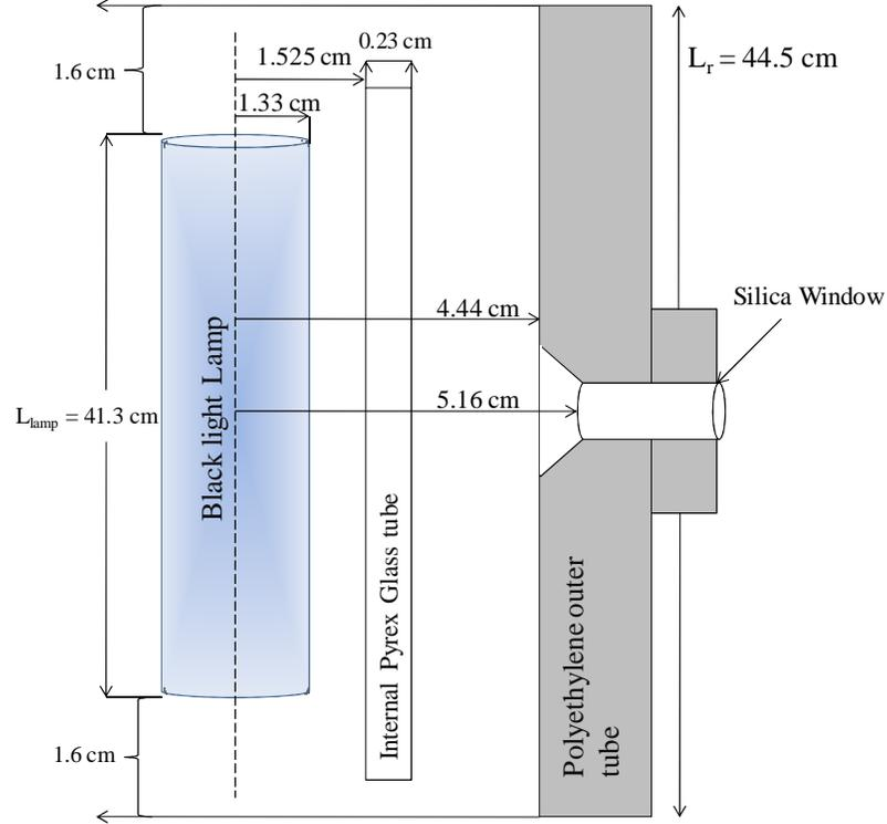
**Figure 24** Dimensions for the Photo-CREC Water-II photoreactor
