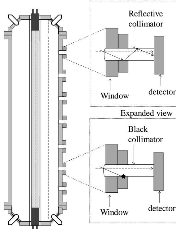
**Figure 11** Detailed view of the sensor collimator arrangement
