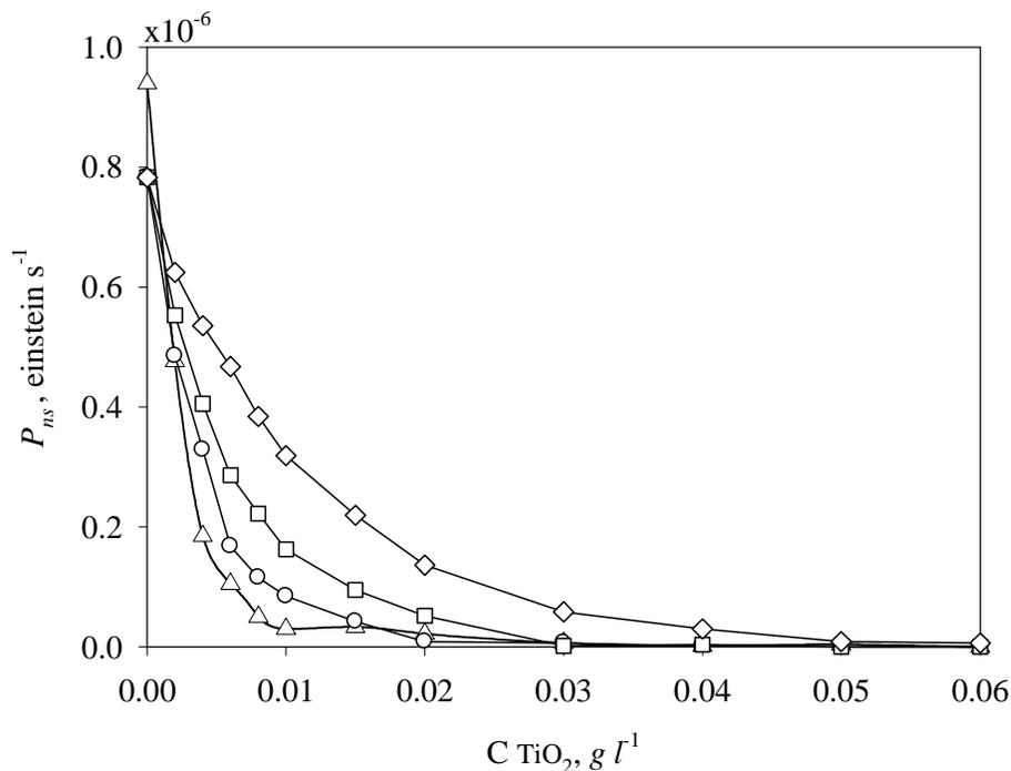
**Figure 20** Transmitted non-scattered radiation vs. catalyst concentration expressed in einstein s<sup>-1</sup>. (Δ) DP 25, (○) Anatase, (□) Hombikat UV-100 and (◇) Sol-Gel Cat
