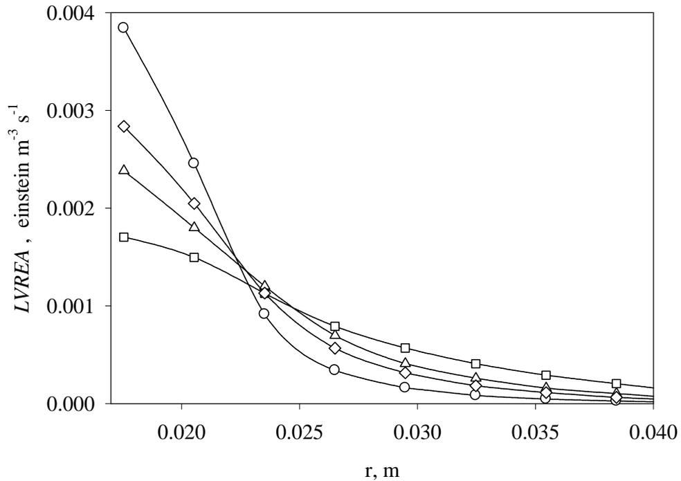
**Figure 30** Radial profiles of LVREA for different DP 25 concentrations by MC. ( $\circ$ ) 0.14, ( $\diamond$ ) 0.09, ( $\Delta$ ) 0.07 and, ( $\square$ ) 0.04 g l<sup>-1</sup>
