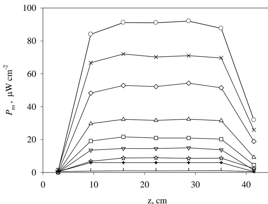
**Figure 18** Axial distribution of the radiation transmission in the photoreactor when  $\text{TiO}_2$  DP 25 and black collimator are used. (○) 0, (×) 2, (◇) 6, (△) 10, (□) 15, (▽) 20, (☆) 30, (+) 50 and (|)  $90 \text{ mg l}^{-1}$
