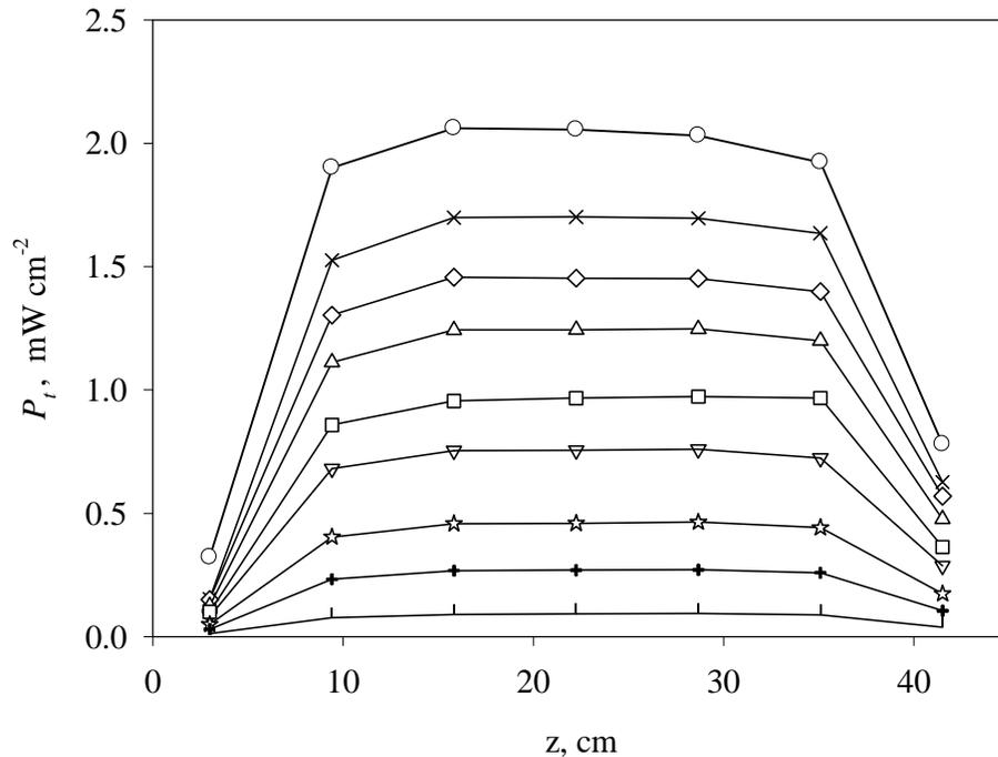
**Figure 17** Axial distribution of the radiation transmission in the photoreactor when  $TiO_2$  DP 25 and aluminum collimator are used. (○) 0, (×) 2, (◇) 6, (△) 10, (□) 15, (▽) 20, (☆) 30, (+) 50 and (l) 90  $mg\ l^{-1}$
