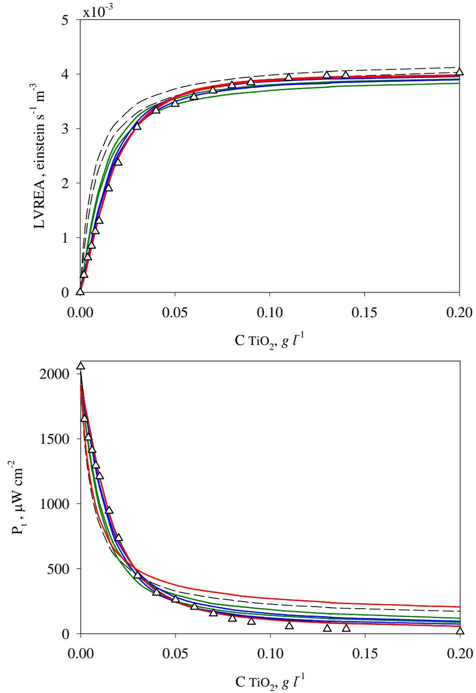
**Figure 29** Asymmetry factor influence in MC simulation 4, ( $\Delta$ ) experimental results for DP 25, (---)  $g = 1$ , (---)  $g = -1$ , (green —)  $g = 0.8$  and  $-0.8$ , (blue —)  $g = 0.5$  and  $-0.5$  and (red —)  $g = 0.1$  and  $-0.1$
