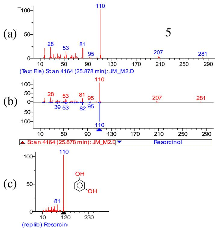
Figure A-7 Mass spectrum for component 5, Resorcinol
