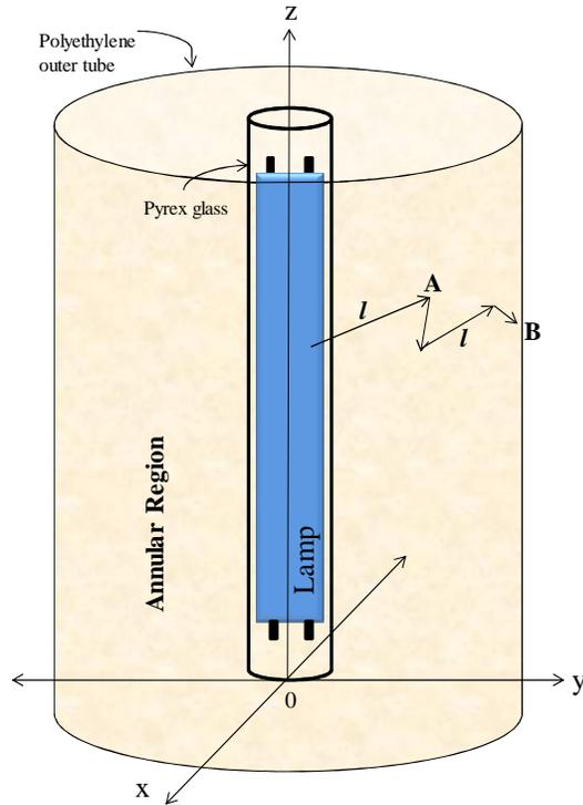
**Figure 23** 3D view of the annular region used for MC simulations
