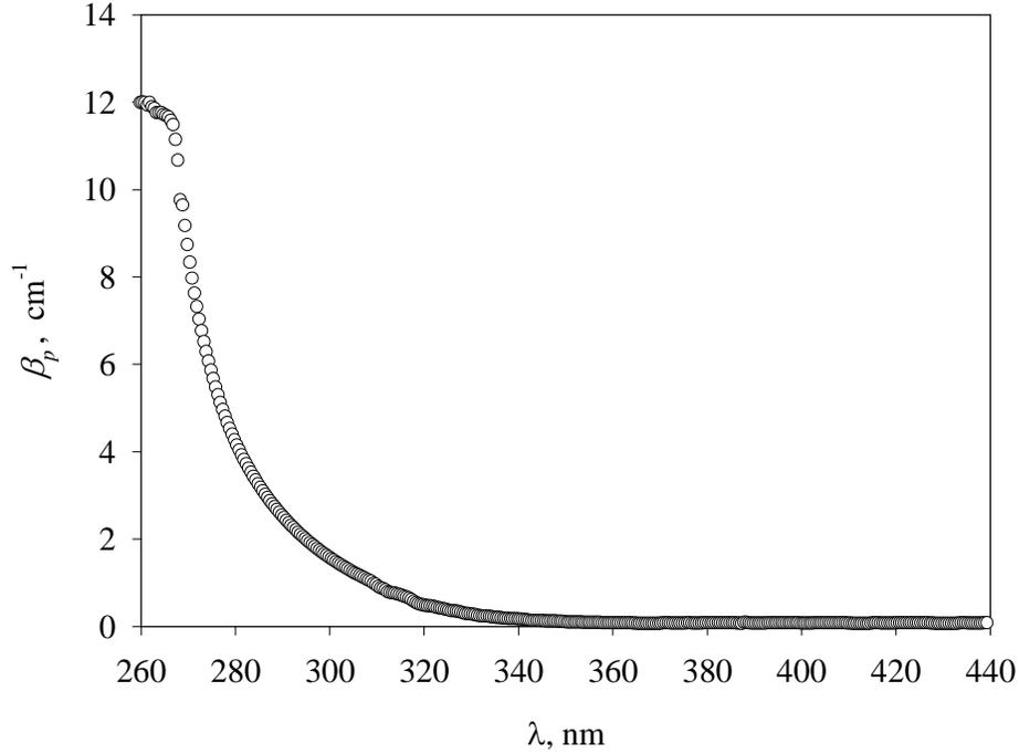
**Figure 16** Extinction coefficient of the Pyrex glass
