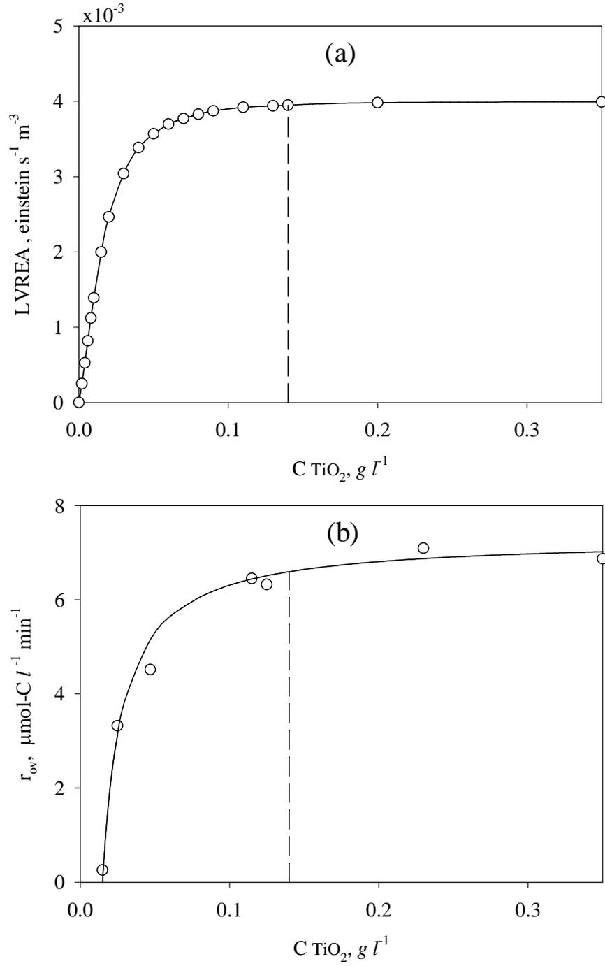
**Figure 31** (a) LVREA inside the Photo-CREC Water-II as a function of DP 25 loading. (b) Overall reaction rate for phenol degradation versus DP 25 concentration (as presented by [Salaices et al., 2001](#))
