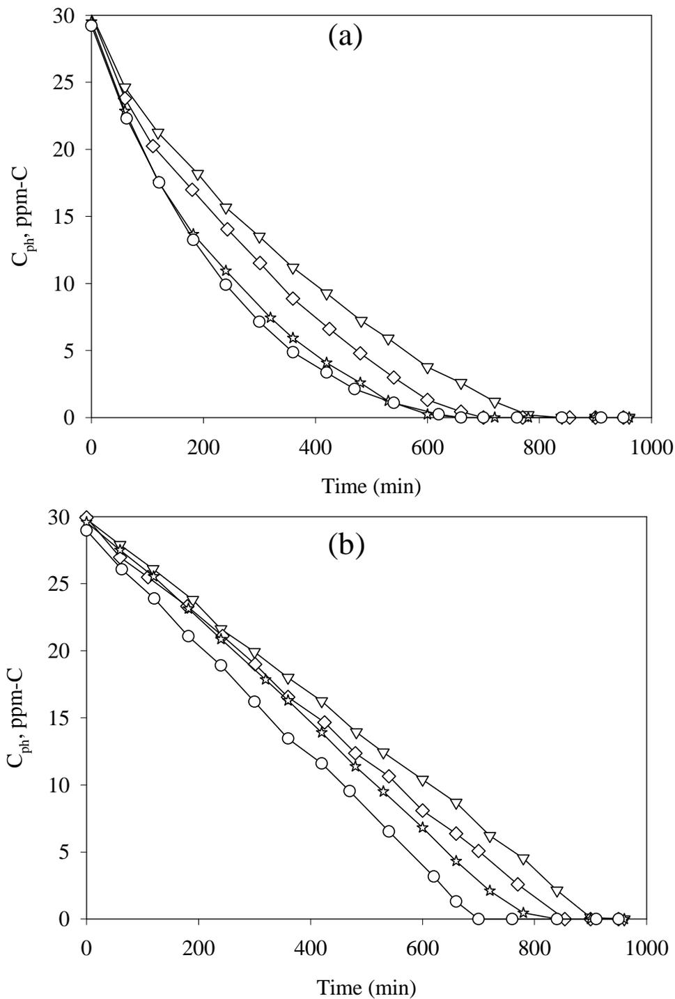
**Figure 53** Influence of iron ions on the photocatalytic degradation of phenol (a) phenol and (b) TOC profiles for ( $\nabla$ ) DP 25, ( $\star$ ) DP 25+Fe<sup>3+</sup> in solution, ( $\diamond$ ) Sol-Gel Cat, and ( $\circ$ ) Sol-Gel Cat+Fe<sup>3+</sup> in solution
