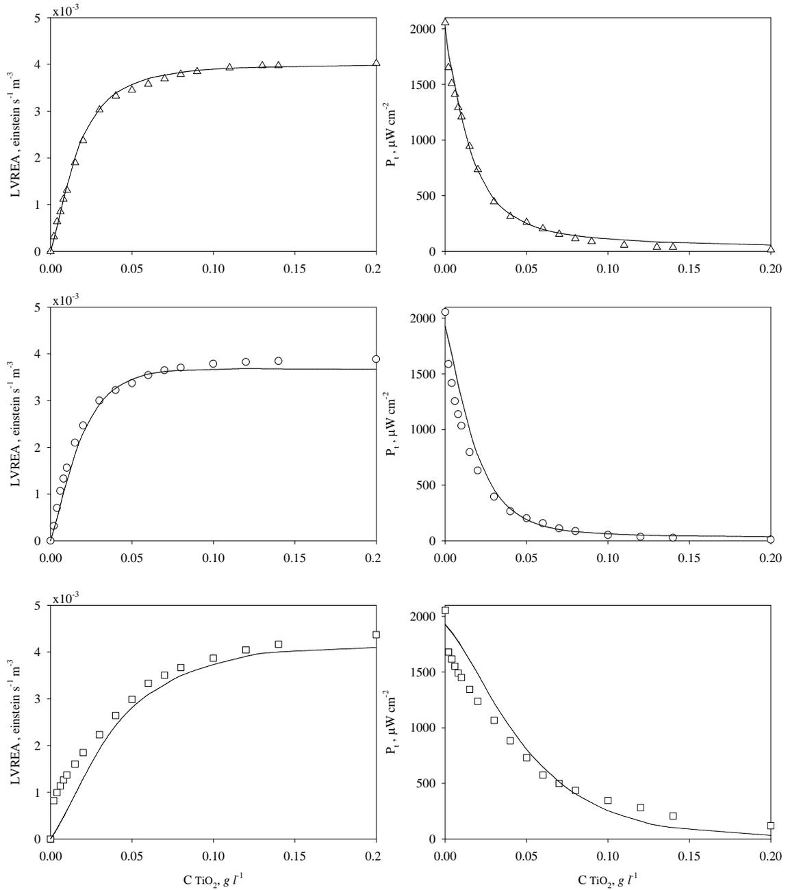
**Figure 28** Experimental results for the LVREA, and the transmitted radiation and comparison with “MC simulation 3”. Experimental data: ( $\Delta$ ) DP 25, ( $\circ$ ) Anatase, and ( $\square$ ) Hombikat UV-100 and (—) MC simulations
