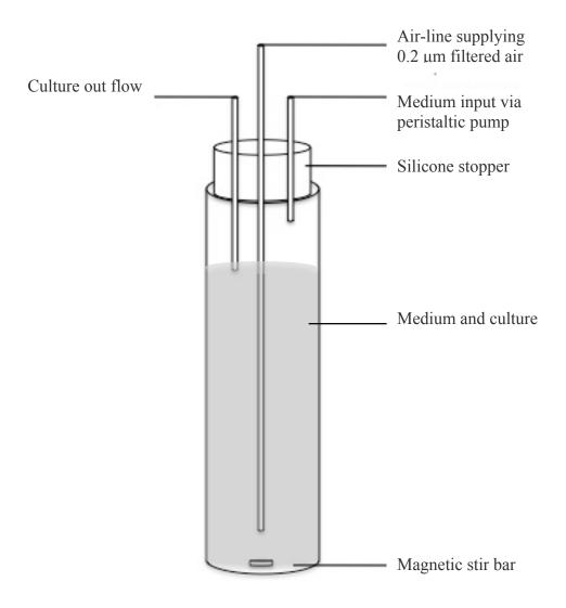
Figure 5.1 Chemostat experimental set up.
