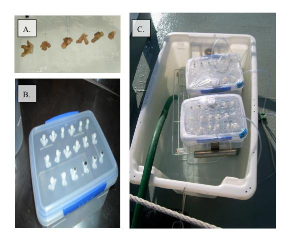
**Figure 4.2** Experimental chamber set up. *S. pistillata* nubbins were cut from colony fragments and suspended on monofilament line (A.). Eighteen nubbins were placed into 4L trace metal-clean containers (B.) and placed into a flowing seawater bath (C.).
