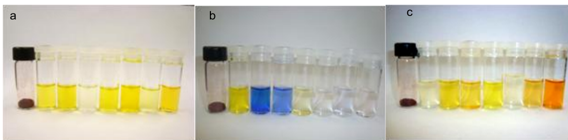
Figure 3-9: Compound III-3 in a) various solvents: from left to right: dioxane, dichloromethane, chloroform, diethyl ether, methanol, ethanol and \text{H}_2\text{O} . b) after addition of TFA., c) after basification.
