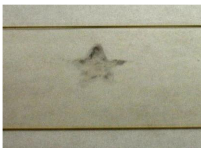
Figure 6.7 AuNPs patterned on a piranha-treated glass slide utilizing photoinitiated carbene insertion method.
