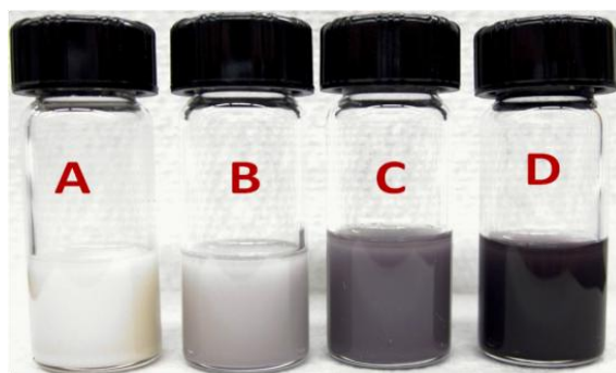
Figure 5.5 Photograph of the following suspensions in THF; A) Fenton- treated micro-diamond B) Fenton-treated micro-diamond after dark/control reaction C) Diamond-AuNP hybrid prepared using as-received micro-diamond post-photolysis and D) Diamond-AuNP hybrid prepared using Fenton-treated micro-diamond post-photolysis.
