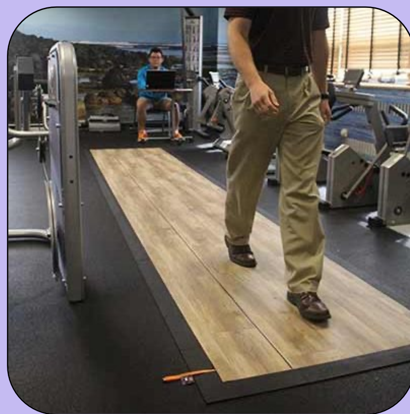
Fig. 1. Example of a Zeno™ Walkway 4 . Gait is recorded in the thicker segment of the mat (right in the image) and is not recorded in the thinner strip or on the black border.
