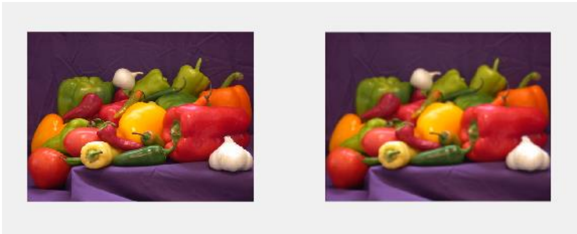
Figure 7: An example of image convolution, where the input image was smoothed used a convolutional filter. The gaussian blur filter is used implemented as a 3x3 matrix of values. During the numerical convolution this results in the right blurred image.
