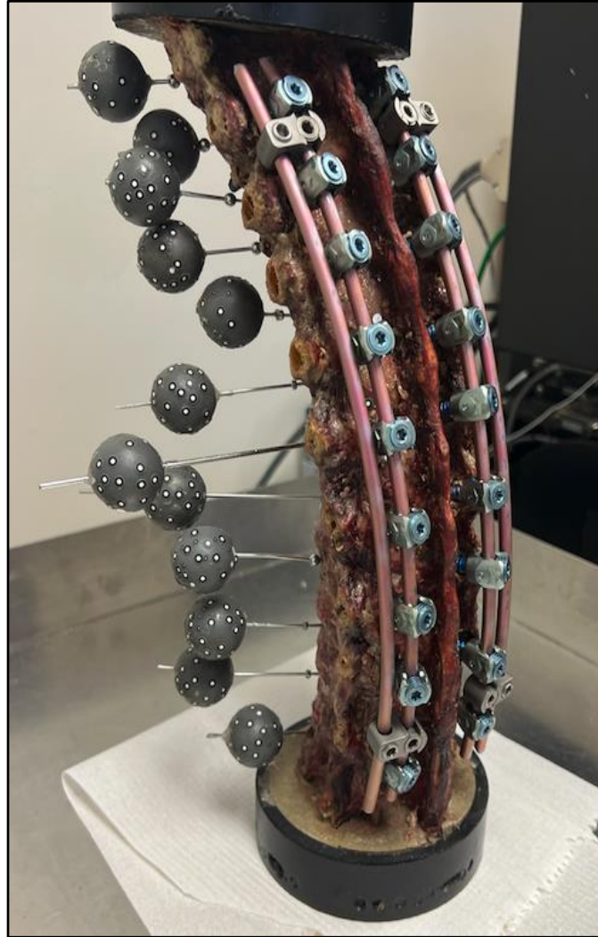
Figure 6. Attachment of markers for digital image correlation system
