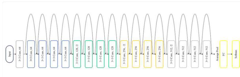
Figure 2.6. Original ResNet18’s architecture
