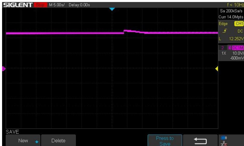
**Figure 4.16.** The bus voltage after sudden disconnection of 30W load (0-70sec)
