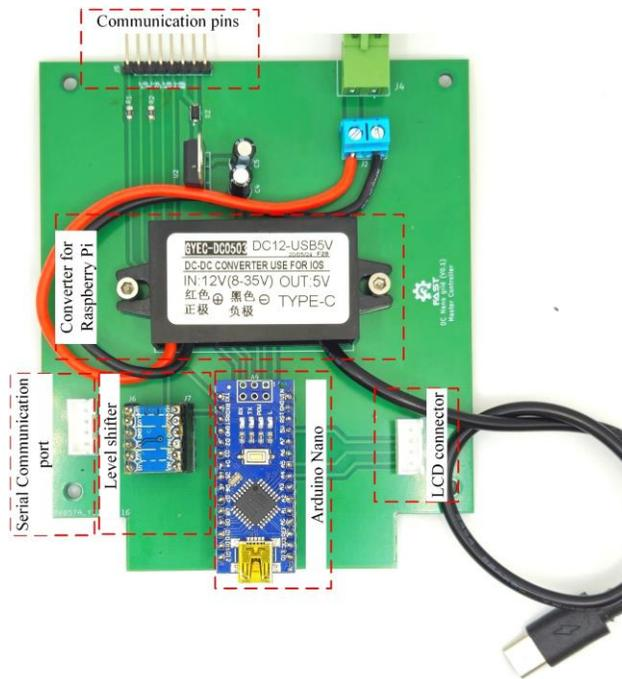
**Figure 4.11.** Master controller PCB layout and assembly.
