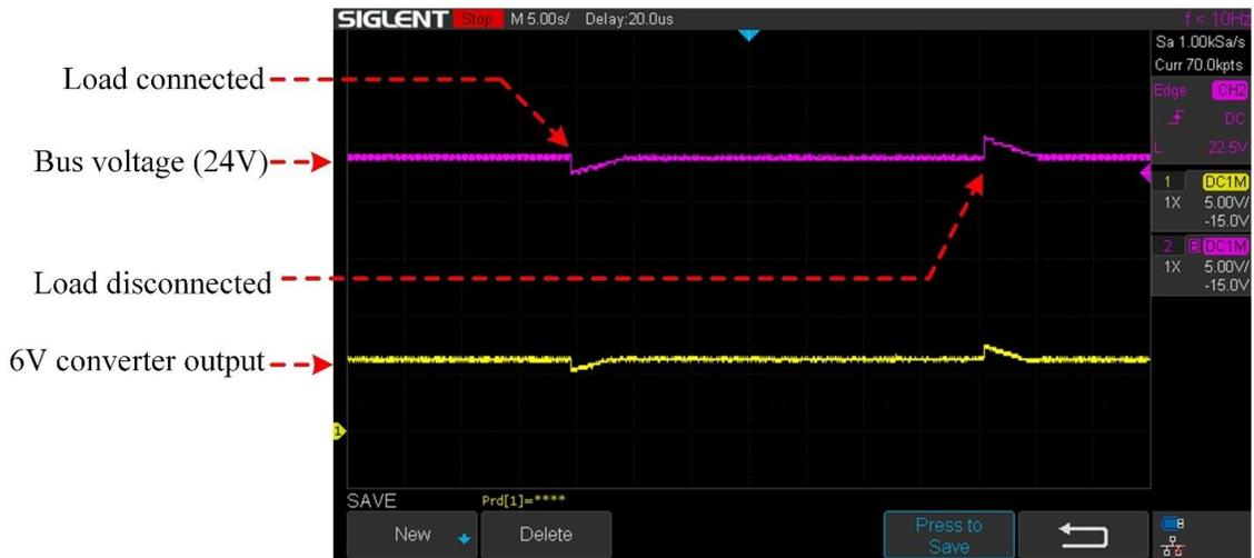
**Figure 5.13.** Bus voltage and 6V converter voltage variation due to load change (0-70sec)
