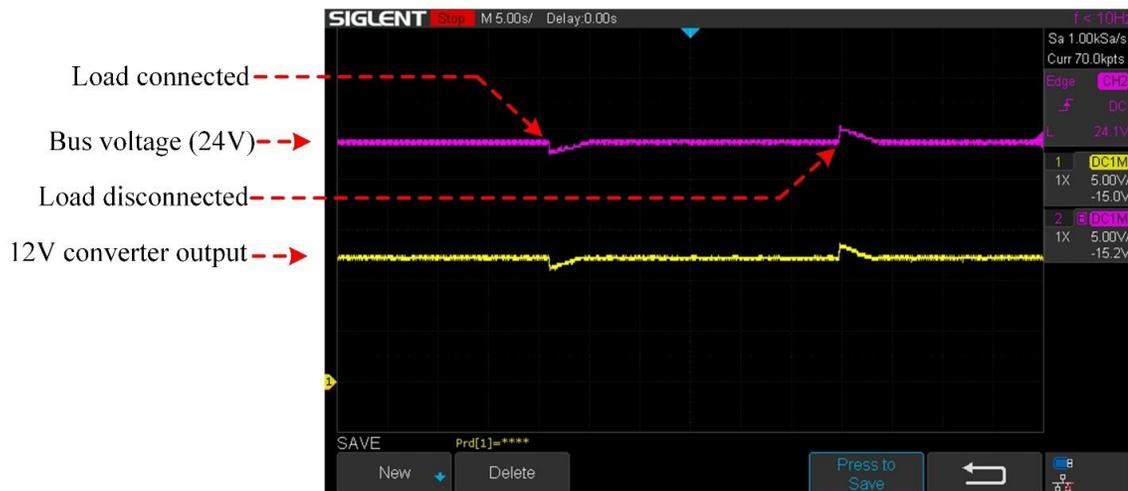
**Figure 5.14.** Bus voltage and 12V converter voltage variation due to load change (0-70sec)
