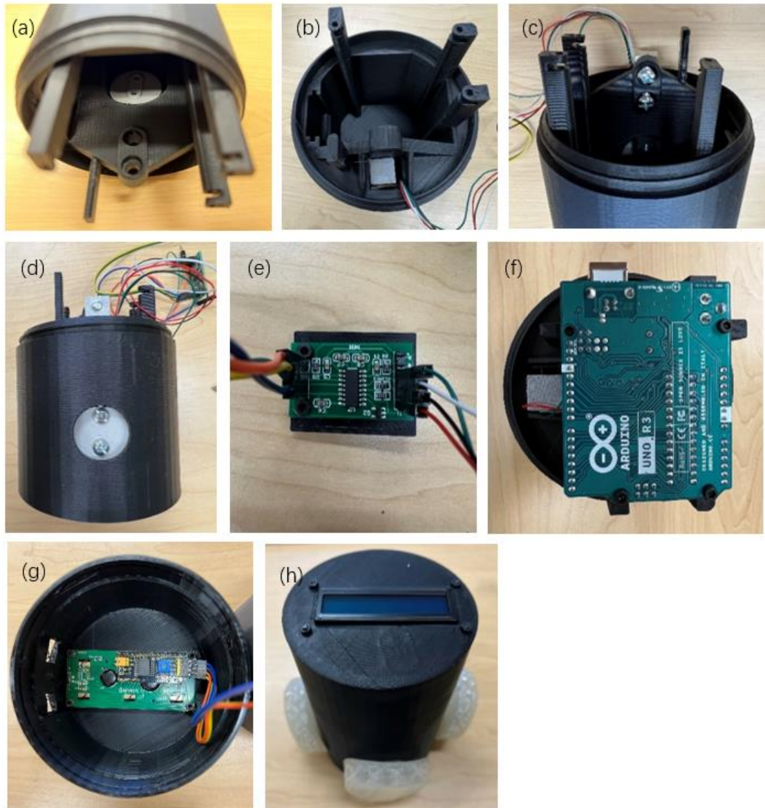
Figure 43. Assembly steps of physical components. (a) Put the flat part into the groove, (b) Insert the load cell, (c) Fix the load cell, (d) Fix the flat, (e) Fix the amplifier, (f) Fix the Arduino Uno board, (g) Fix the LCD on the cap, and (h) Insert the TPU button.
