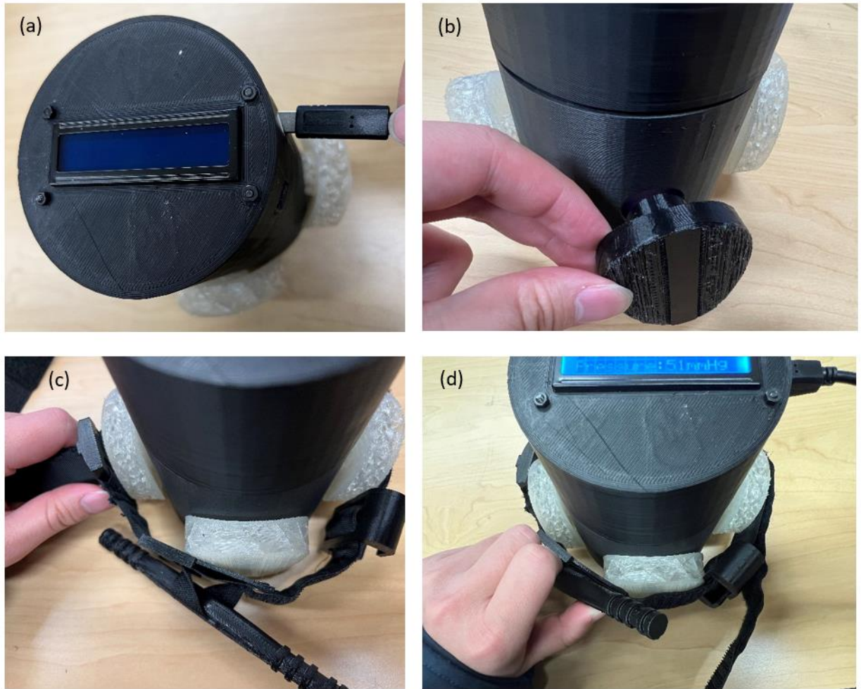
Figure 10. Measurement process (a) Plug in the power cord (b) Insert Tournbutton-M (c) Wrap the tourniquet to the tester (d) Turn the tourniquet windlass.
