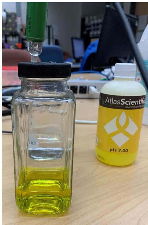
Figure 3.29: pH Sensor Calibration with pH 7.00 Solution
