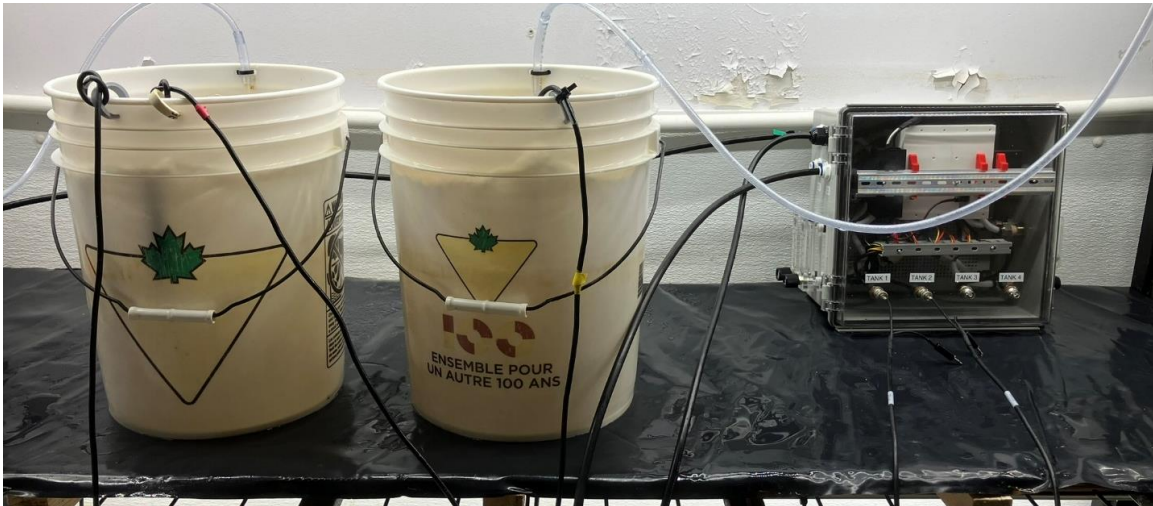
Figure 4.15: Experimental Setup (Left: Tank 1, Middle: Tank 2, Right: BREAD Controller)
