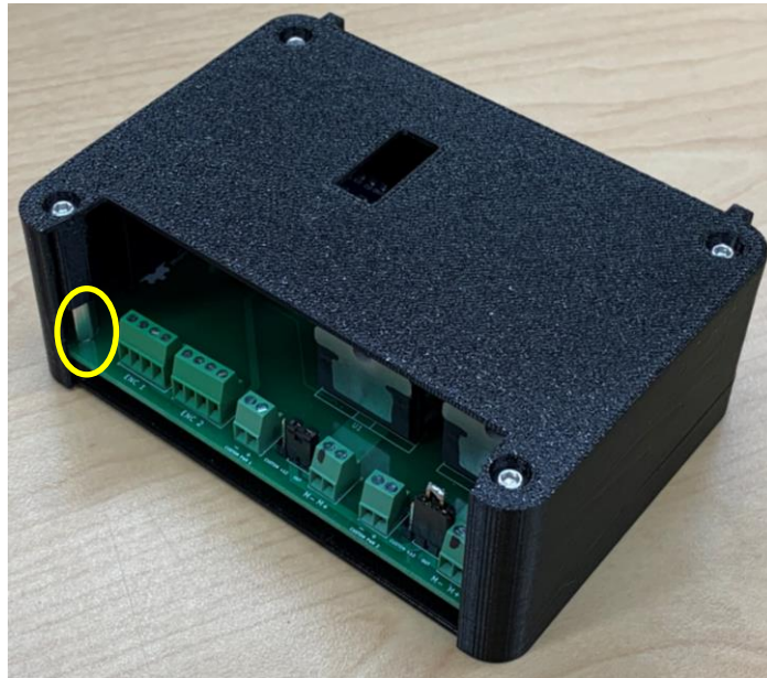
Figure 3.16: Assembled SLC_DCMT with Hex Standoff (circled in yellow)
