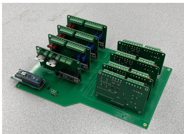
Figure 1.1: BREAD Iteration 1: Pyrolysis Reactor Controller
