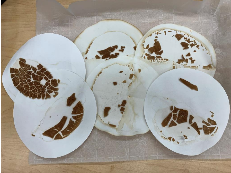
Figure 3.37: Dried yeast samples (Samples were dried on a desktop 3D printer build plate set to 50°C)
