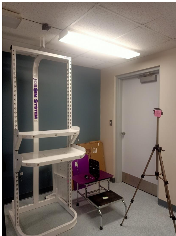
Figure 2-4. Test setup prepared for the study including the Job-Sim settings and Go-Pro Cameras
