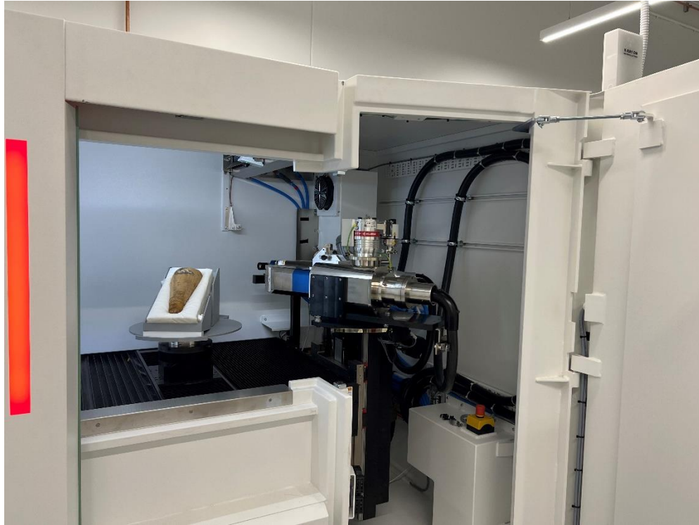
Figure A.12 The photograph shows the mounting and positioning of ibis 2727.01 within the Xylon FF25 CT scanner. Concurrently, the door of the scanning apparatus is opened, exposing the X-ray tube.
