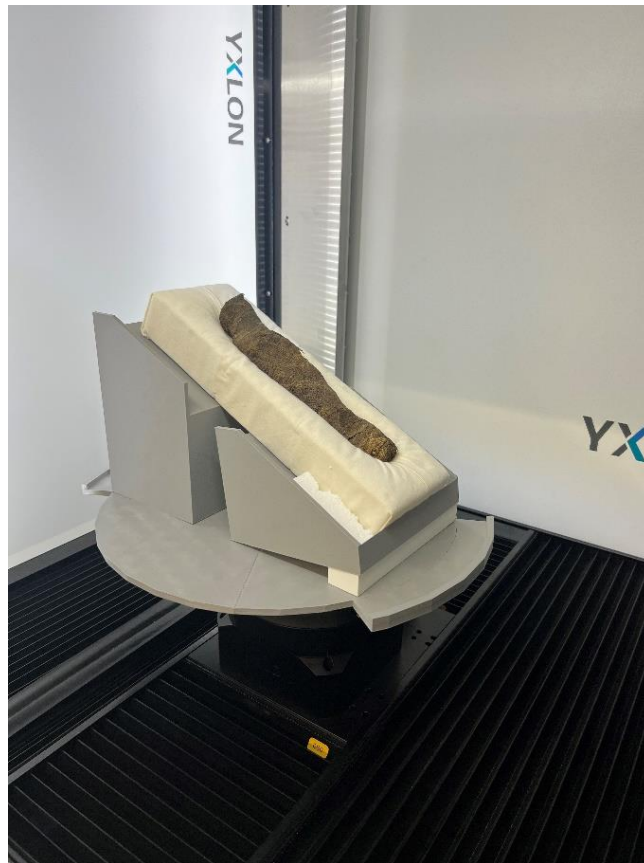
Figure A.1 Demonstrates the mounting and positioning of faucon 5731 in the Yxlon FF25 CT scanner.
