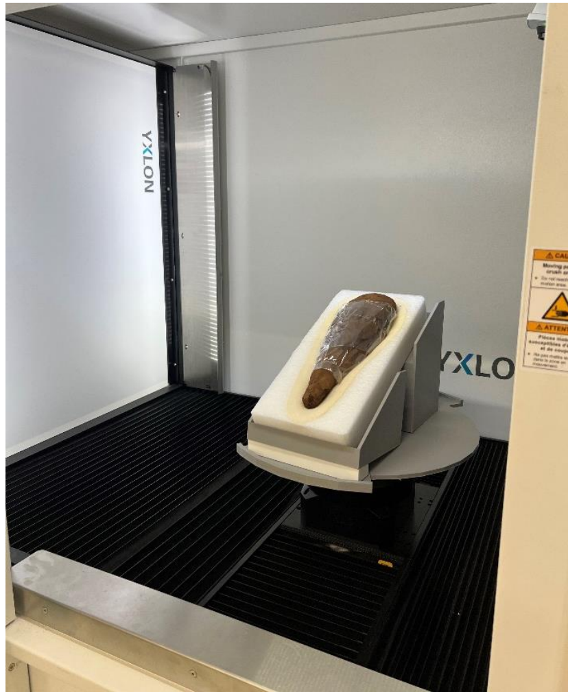
Figure A.7 Depiction of the mounting and positioning of ibis 2727.02 within the Yxlon FF25 CT scanner.
