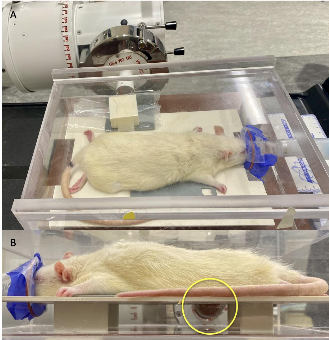
Figure 5. Positioning of a rodent on the 3D printed “Rat-form” showing the targeting of the Orthovoltage unit 3cm cone centered at the implant and fat-pad which lies below the rest of the rats body highlighted by the yellow circle (B).
