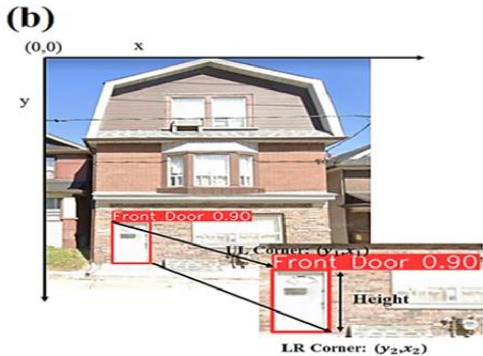
Figure 3-2: a) FFH definition b) GSV pixel size estimation in y-direction; 0.9 refers to the bounding box confidence value; UL and LR stands for the Upper Left and Lower Right corners
