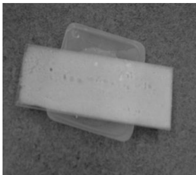
Figure 4.2: TiO 2 -PVP photocatalyst immobilized on a glass slide
