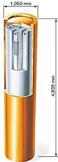
Figure 2.1: SKB's reference canister with an outer corrosion barrier of copper and an insert of nodular cast iron (With permission of SKB) [4,5].
