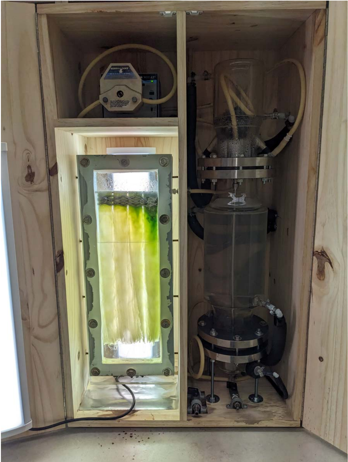
Figure G Benchtop algae recirculation bioreactor.
