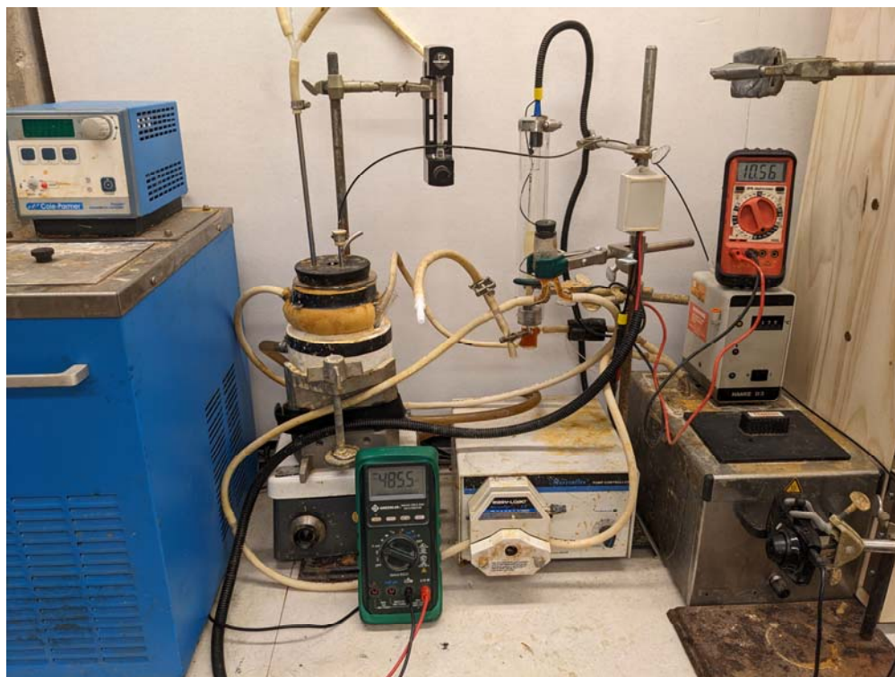
Figure F BioGenerator broth oxygen solubility measurement apparatus.
