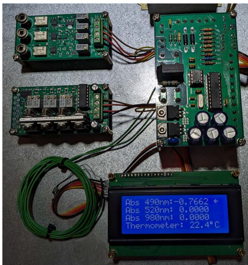
Figure 4.13 Prototype spectrophotometer for monitoring of the BioGenerator broth.
