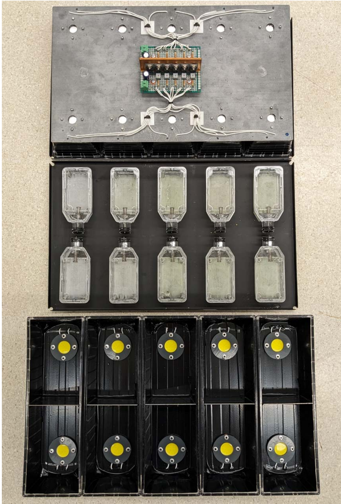
Figure H Algae growth dishes and illuminating caddy (exterior and interior view).
