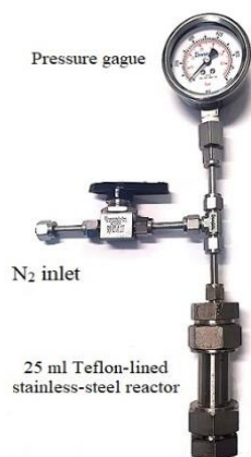
Figure 4.2: Schematic of the reactor used for the hydrolysis reaction.
