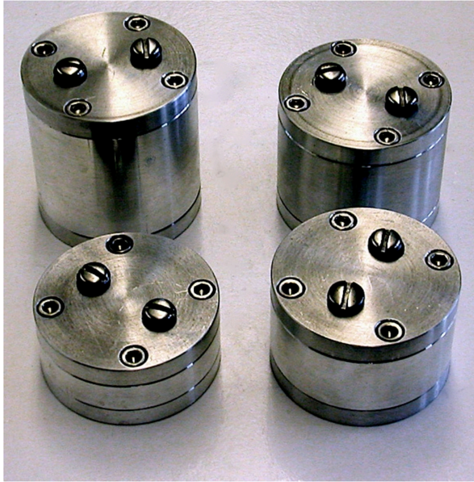
Figure 2.1: Moulds used to produce PVA hydrogel ultrasound phantoms for Prof. Tamie Poepping’s ultrasonics group at The University of Western Ontario, Canada.
