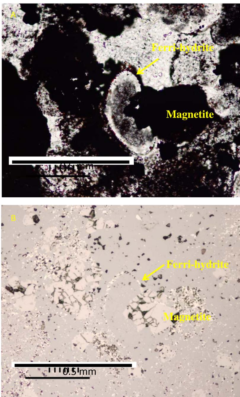
**Plate 3.9: Photomicrograph of a granule rinded by ferri-hydrites in a granular-textured band of sample 26-075-1136 overgrown by blocky magnetite. (A) is in plane polarized light and; (B) is in reflected light.**
