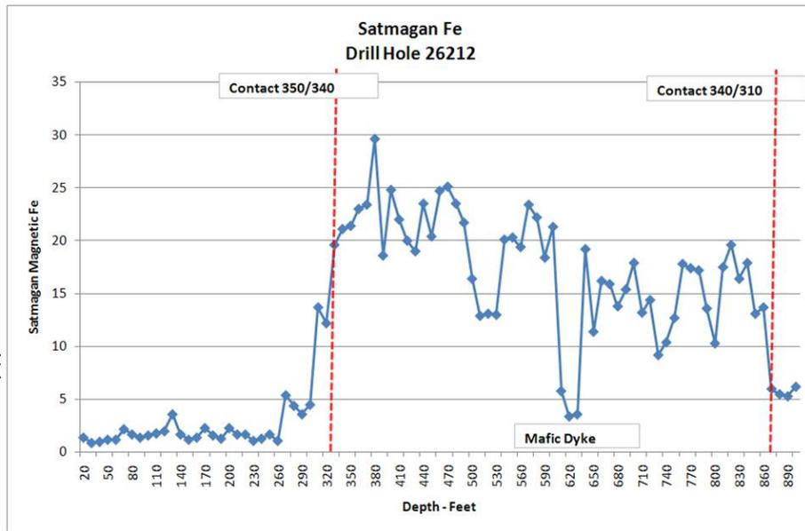
**Figure 3.5: Example of a Satmagan reading down drill hole 26-212 delineating the contact between the Main Pit Carbonate (340) and Martite (350), the Main Pit Carbonate (340) and lower Clastic (310) domains.**
