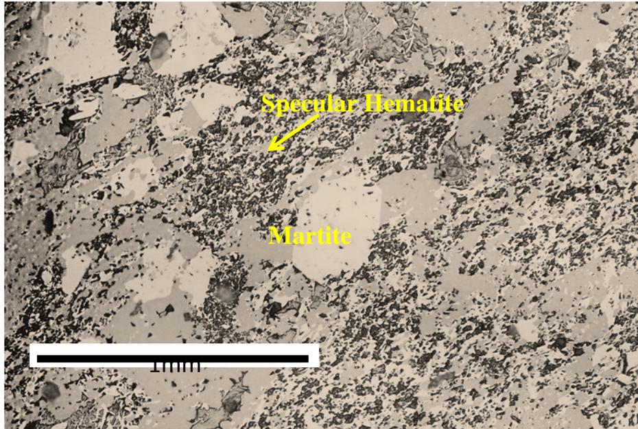
**Plate 3.11: Photomicrograph of the near complete replacement of magnetite by martite and the abundant laths of specular hematite in sample 26-080-614 (reflected light). Note the hematite defines a weak foliation.**
