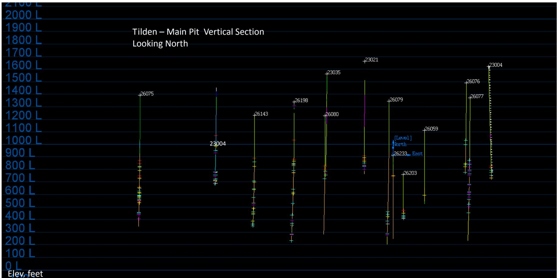
**Appendix B2: Cross-section map. Sample Locations of the drill holes investigated in this these. Elevations relative To sea level are marked by the blue numbers on the left side of the diagram. The X,Y and Z co-ordinates are listed in the Sample List of Appendix B.**
