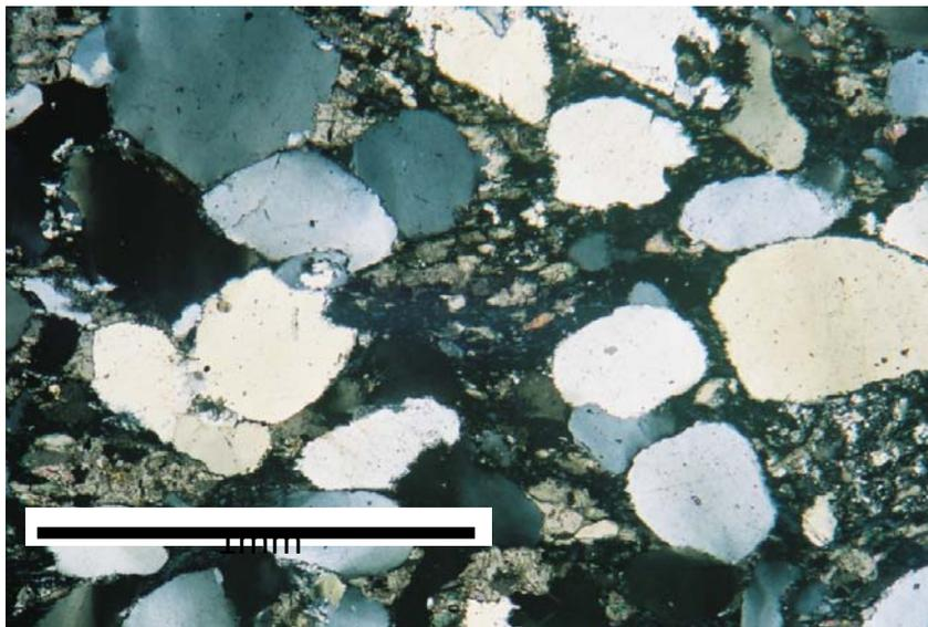
**Plate 3.2a: Photomicrograph in cross polarized light of coarse grained clastic texture in sample 26-077-1119. Detrital quartz grains display strained extinction. Late carbonate, chlorite and magnetite are interstitial to the quartz grains.**
