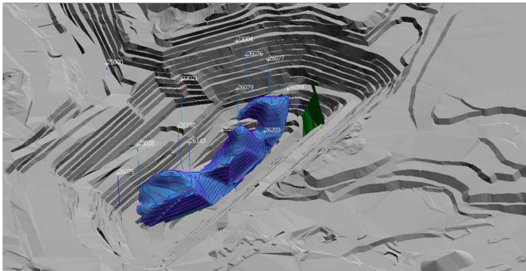
**Figure 3.2: A contour map delineating the top of the Main Pit Carbonate (340) Domain as it is identified in the pit in contact with the overlying Martite Domain. Drill holes used in the current research are labelled with white numbers. The green plane represents the location of the Tower Fault. Map courtesy of Cliffs Technical Staff.**
