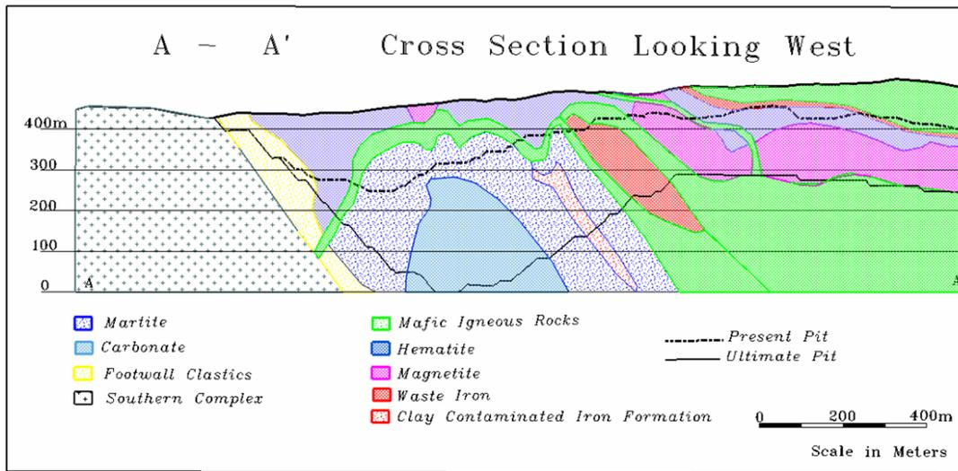
**Figure 3.0: A stratigraphic cross-section (A-A' of figure 2.6) that illustrates the anticline as defined by mapping of the igneous “Pillar” marker. The southern limb of the anticline has a steeper dip than the northern limb and is truncated by the sheared contact with the Southern Complex. The Main Pit Carbonate and Martite Domains are located beneath the igneous Pillar (Scott and Lukey, 1999).**
