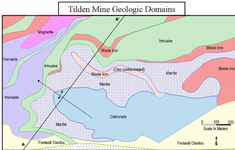
**Figure 3.1: A generalized geology map of the domains defined by the Tilden technical staff. The Main Pit Carbonate and Martite Domains are the focus of the thesis. Note the shallowly plunging northwest anticline delineated by the igneous Pillar horizon (Scott and Lukey, 1999).**
