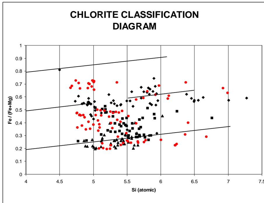
**Figure 4.1: Classification diagram after Zane et al., (1998) depicting the chlorite species of the Basal Clastic Facies (red dots). Note that other symbols on the chlorite classification diagrams are: squares represent Medial BIF, triangles represent Upper GIF and diamonds represent hydrothermal chlorite.**
