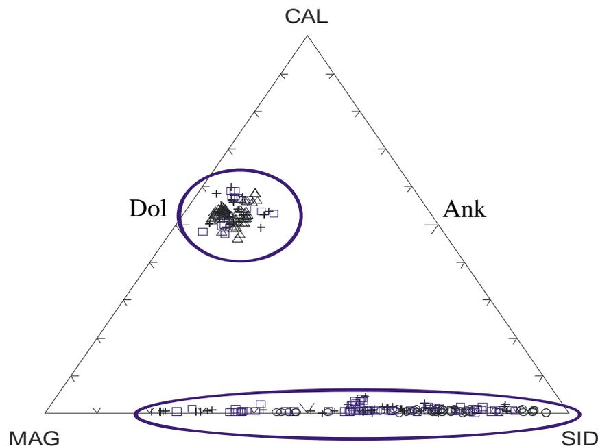
**Figure 4.5:** A ternary diagram after Chang et al., (1998) of the two different carbonate groups (magnesite-siderite and Fe-dolomite-ankerite) within the Medial BIF Facies. Other symbols are: circles represent Basal Clastics, triangles represent Upper GIF and crosses represent initially determined hydrothermal carbonates. The high Mn component is attributed to late hydrothermal carbonates.
