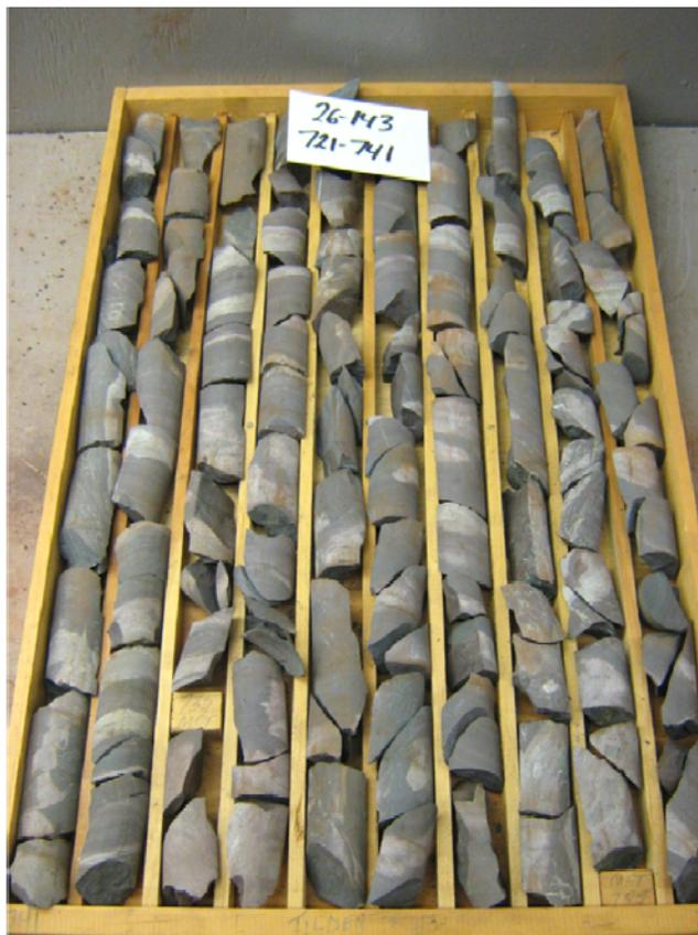
**Plate 3.13: The Upper GIF Facies in drill hole 26-143-(721-741). Note the bleached areas of chert replaced granules and the occasional chert bands.**
