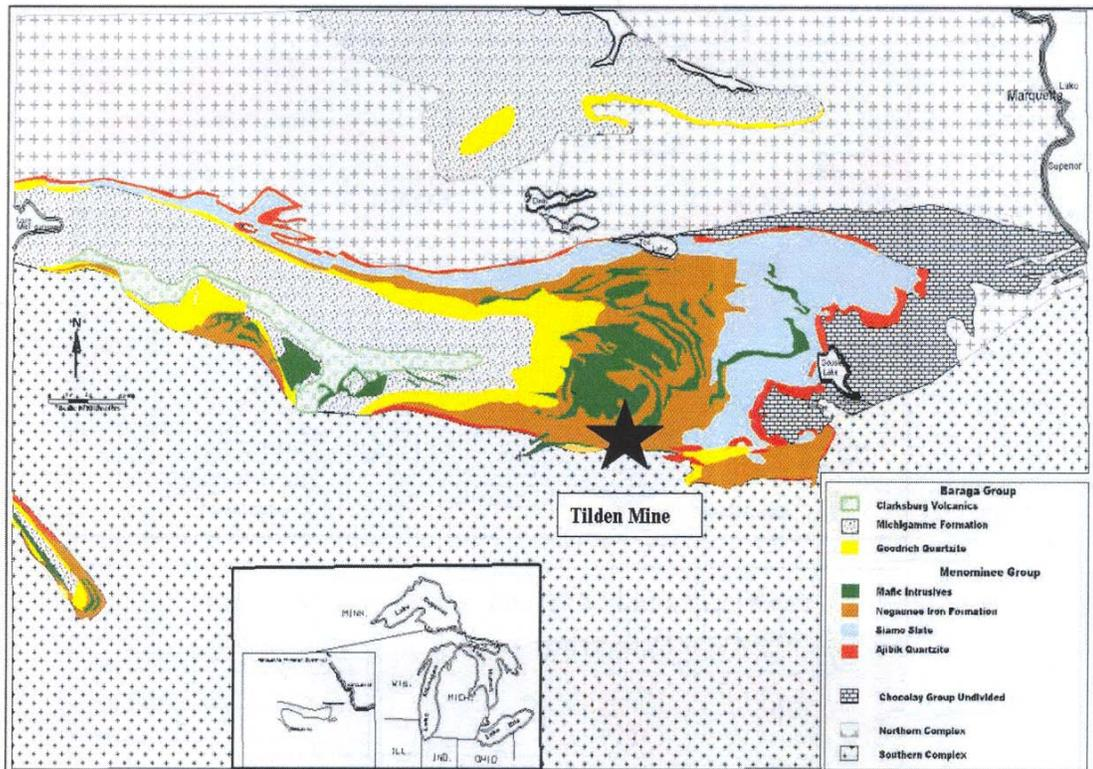
**Figure 2.5: A generalized geology map of the Marquette Range Supergroup in contact with the Southern Complex. The Tilden Mine is located on the contact between the Negaunee Iron Formation (brown) and the Southern Complex (cross-pattern) (Lukey et al., 2007).**
