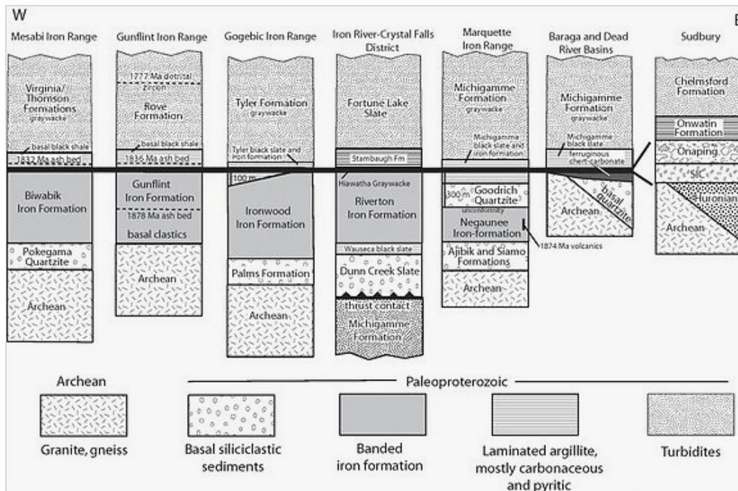
**Figure 2.3: Cross section correlation by Cannon et al., (2010) illustrating the stratigraphic position of the Sudbury Impact Event layer across the Great Lakes region. Note how the spherulitic layer terminates most iron formation deposition with the exception of the Negaunee.**
