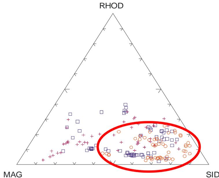
**Figure 4.3: Ternary diagram after Chang et al., (1998) depicting the Mn-rich carbonates of the Basal Clastic Facies. Other symbols are: squares represent Medial BIF, triangles represent Upper GIF and crosses represent initially determined hydrothermal carbonates. The high Mn component is attributed to late hydrothermal carbonates.**
