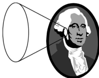
Figure 1.5 An illustration of a cone of confusion. All sound sources located on the surface of this cone produce the same ITD and ILD cues. (Plack 2018)
