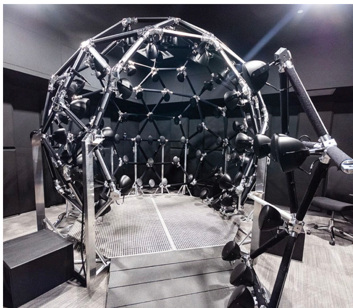
Figure 1.9 The Audio Dome in the sound attenuating chamber at Western University. (A moveable part of the frame rotates around a hinge to provide entrance for the listener. Once closed, the eight channels attached to it complete the spherical structure.)
