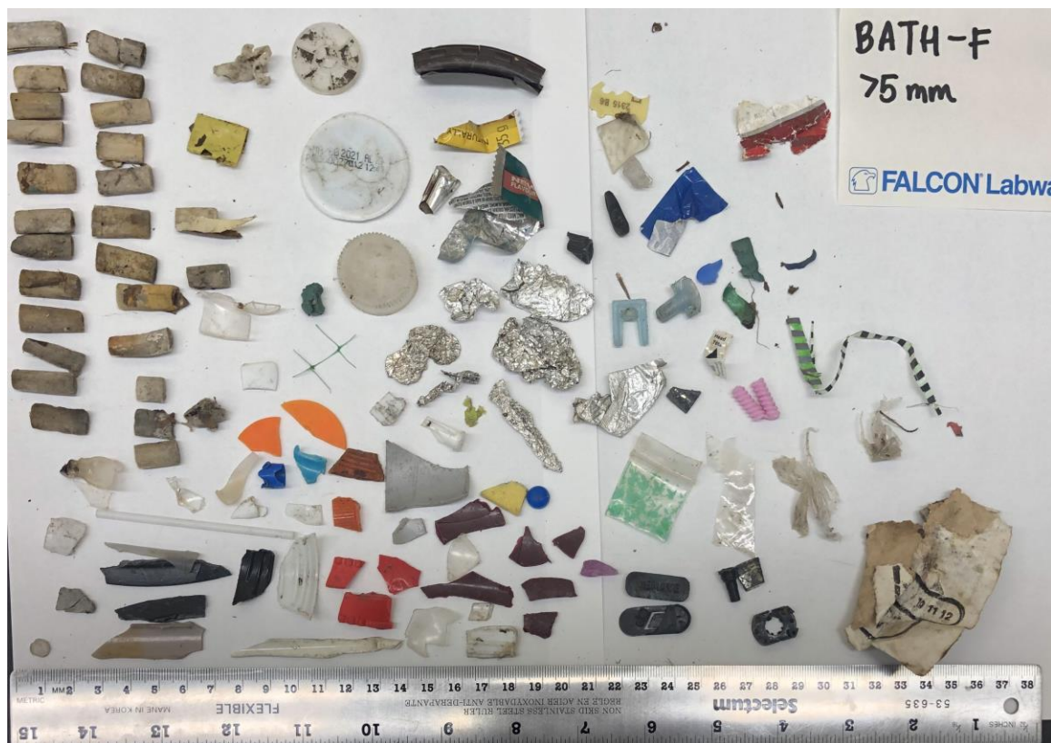
Figure 2-5. Organization of macroplastic and other debris from the autumn Bathurst sample prior to visual characterization.
