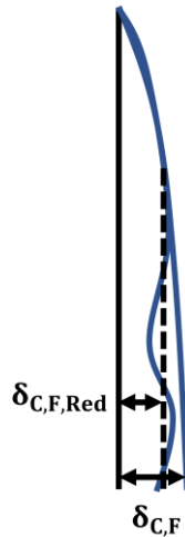
Figure 4.8 Schematic showing reduction of the average condensate film thickness due to the reduction of \delta_{C,F} between the wave-crests. \delta_{C,F,Red} is the reduced value of \delta_{C,F} .
