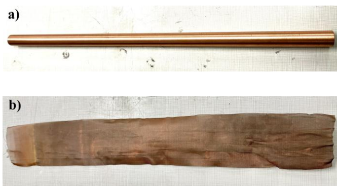
Figure 1.1 a) Prototype of a cylindrical HP. b) Copper mesh wick extracted from a cylindrical HP.
