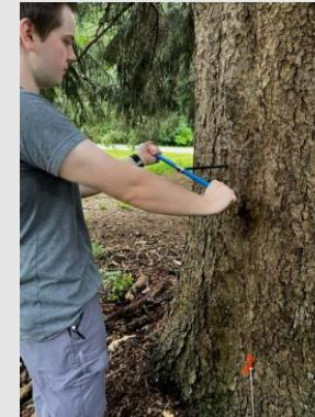
Figure 1. Increment borer used to collect a core from a *Picea abies* tree
