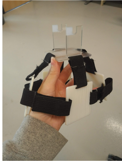
(b) The white squares shown are placeholders for where future gyroscopes could be placed.
