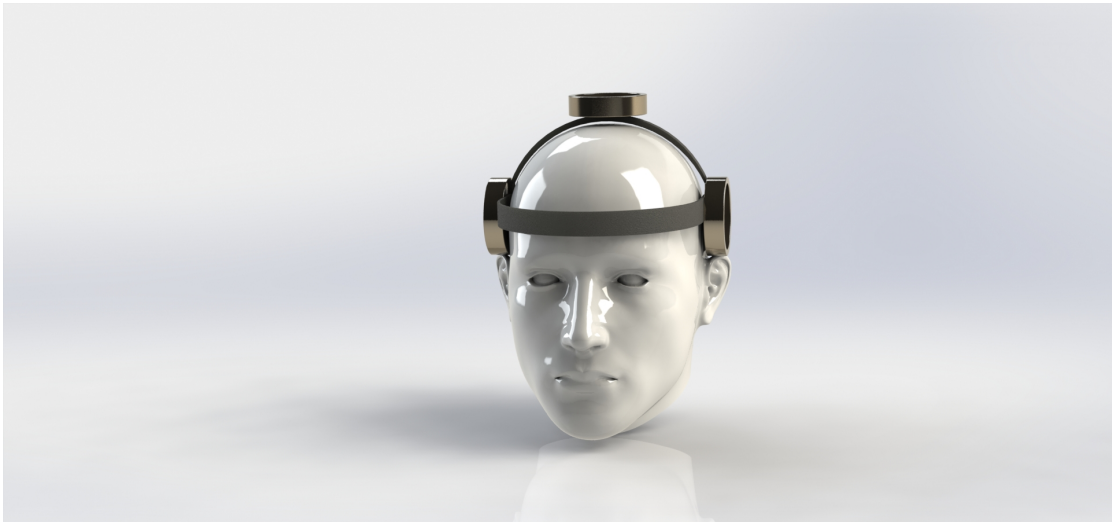
Figure 5.1: A mock up of a first concept for the reaction wheel set up. The initial five wheel design was maintained into the final design. Shown here with the forehead wheel suppressed for a cleaner image.
