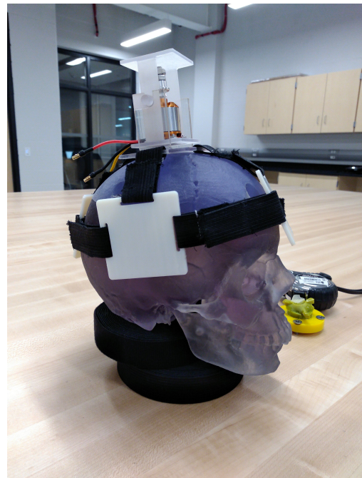
(b) The gyroscope cage seated in the gimbal mount on the harness.
