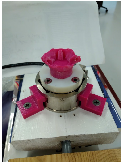
Figure 5.19: The final iteration of the neck mount for the experimental setup—a modified cervical CT scan with only the C1 vertebra (atlas), printed on a pressfit mount to connect to the F/T sensor.
