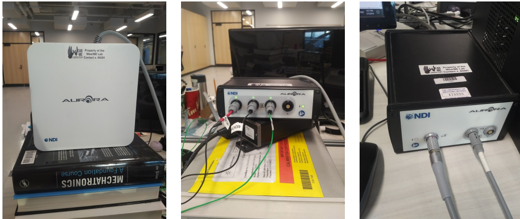
(a) The Aurora Field Generator. (b) The Aurora Sensor Unit. The sensor cables are connected at the front, as shown. (c) Aurora Control System Unit. This connects to the PC, wall outlet, sensor control unit, and the field generator.
