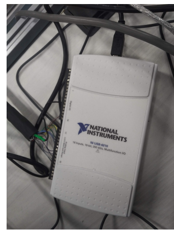
(c) The NI DAQ. Cables wired by experimenter. Connects to the Power Supply (left) and PC (top).
