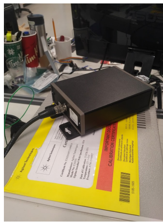
(b) The DAQ Interface Power Supply. Connects to the ATI sensor (left), and the NI DAQ (right) and wall outlet.
