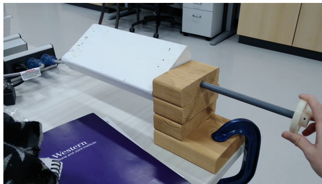
(c) The rotation board assembled, the handle pressfit into the board through the mount.
