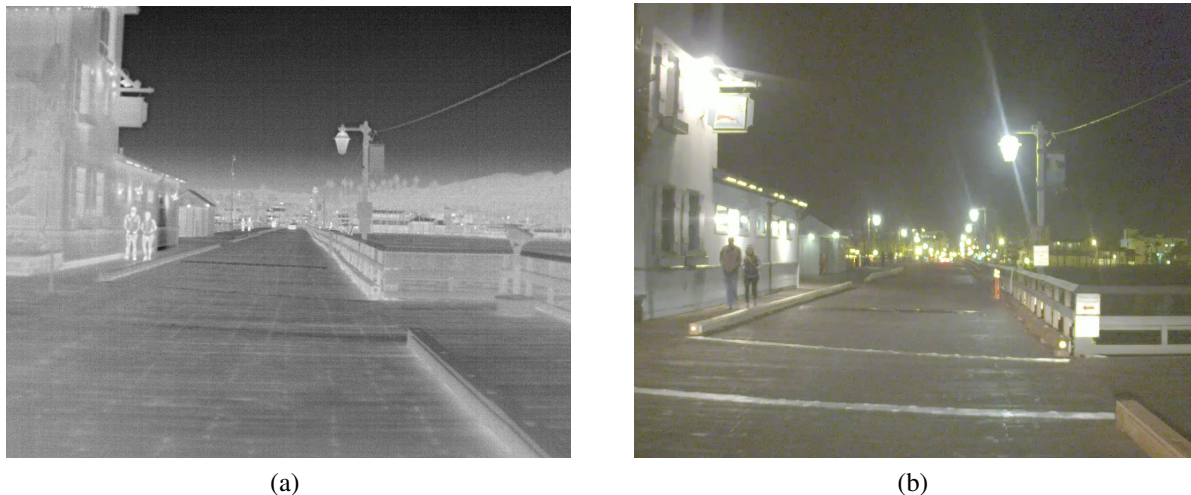
Figure 1.2: Comparison of the same scene captured with a thermal camera (a) and an RGB camera (b) from the FLIR dataset [12]. Thermal image is shown as a grayscale image.
