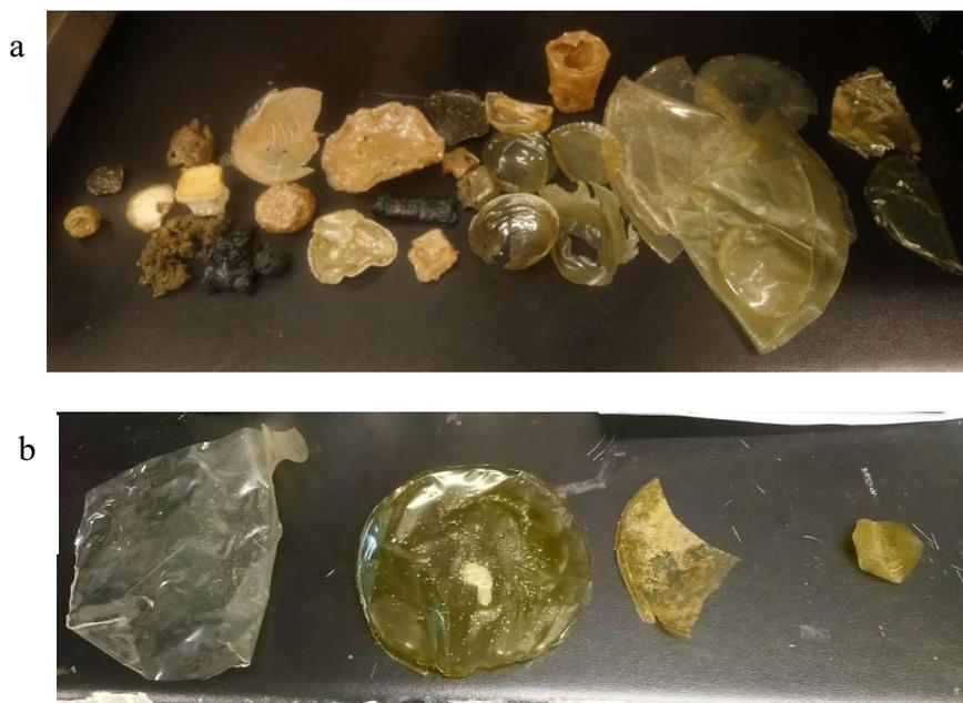
*Figure 4-11a & b: A range of possible biocomposites (a) and films (b) made by varying the ratio of pectin and glycerol*
