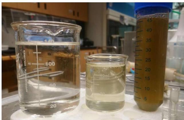
*Figure 4-4: Resulting suspension of combined enzymatic treatment and steam explosion at 500 °C for 15 mins (right)*
