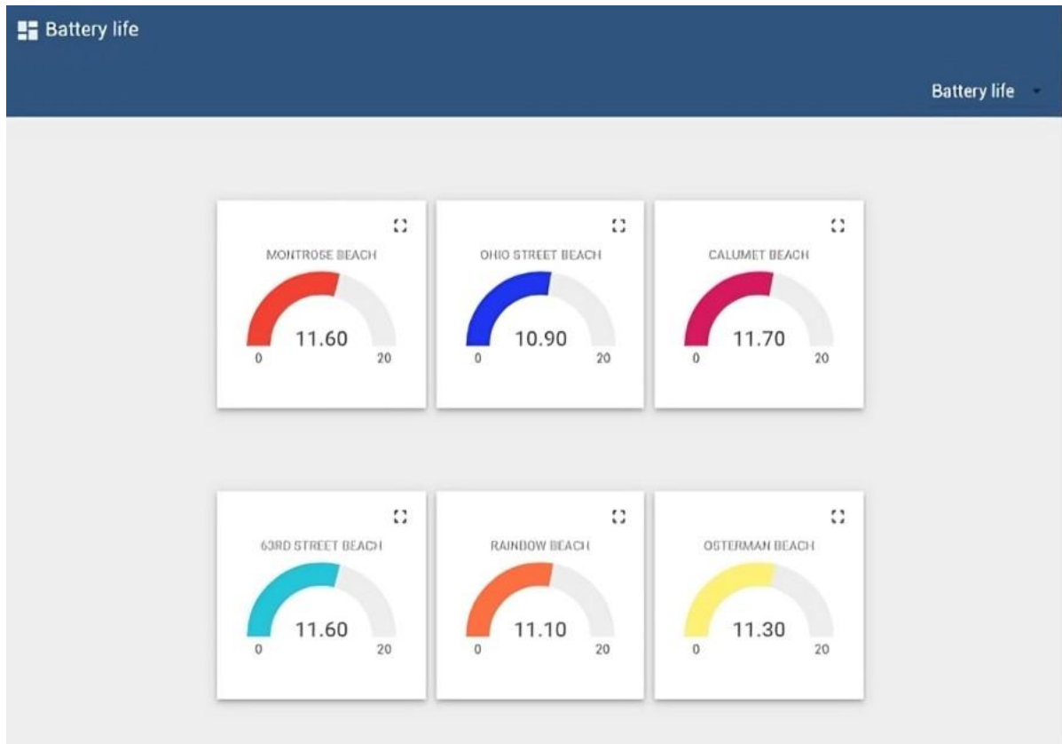
Figure 5.2 ThingsBoard dashboard to show the battery life of the sensors.
