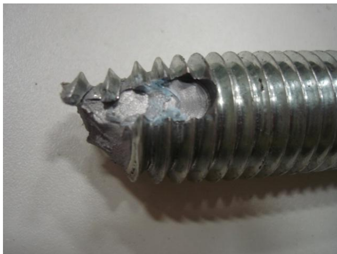
Failure of 3/4" threaded anchor bolt under direct tension (close up)
