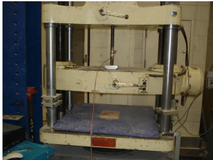
Testing Grade70 – 1" anchor bolt under direct tension test
