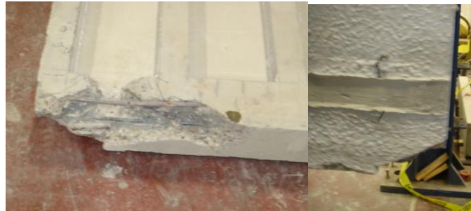
Figure 2.19: Tension anchor side of the joint at the end of the test: front face (left) back face (right)
