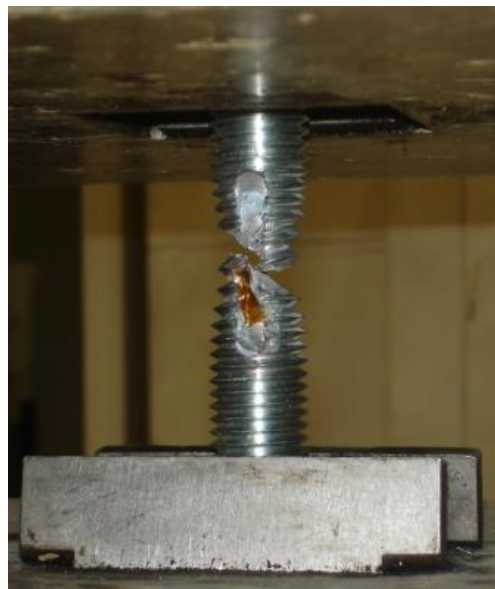
Figure 3.19: Necking, and fracture of a 1" threaded bar under direct tension test
