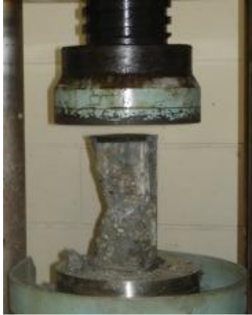
Failure of cylinder under compression test
