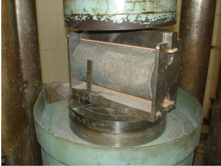
Splitting tensile test
