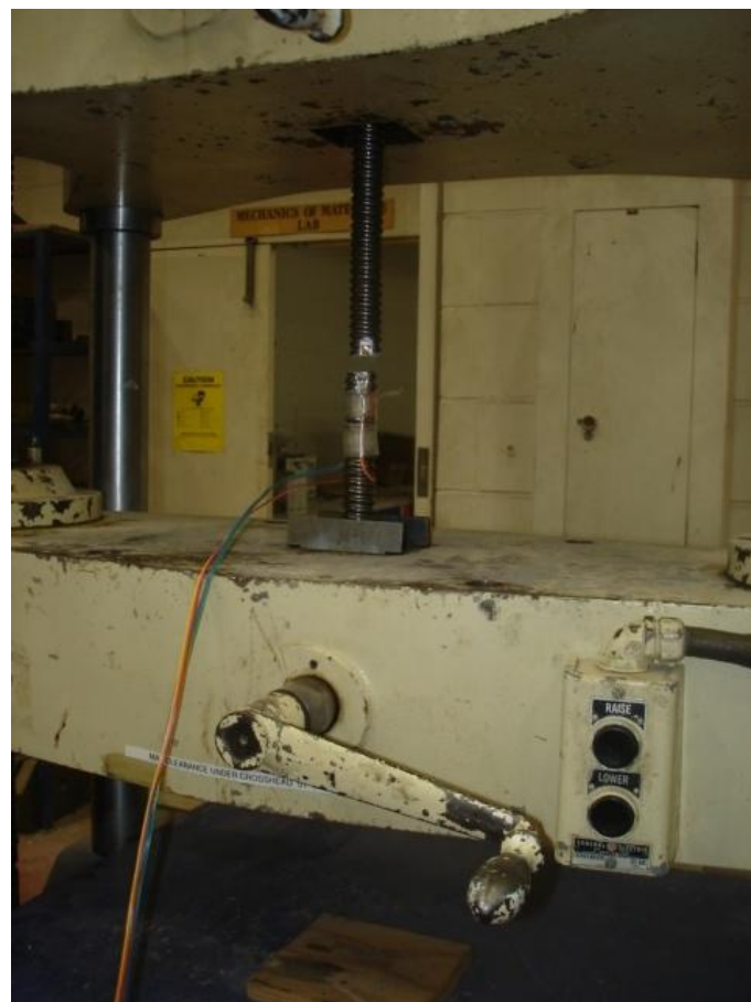
Failure of Grade70 – 1 " anchor bolt under direct tension
