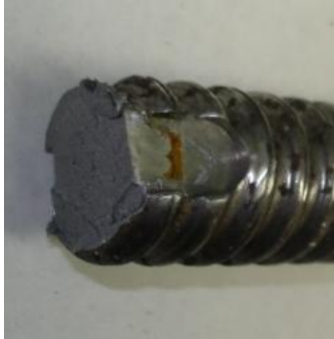
Failure of Grade70 – 1" anchor bolt under direct tension (close up)
