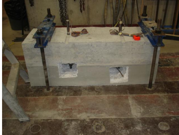
Concrete base block with anchors in place and protruding out
