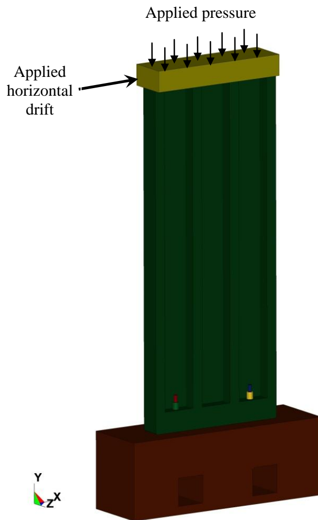
Figure 4.18: Applied pressure to the Anchor-jointed precast structural wall system model
