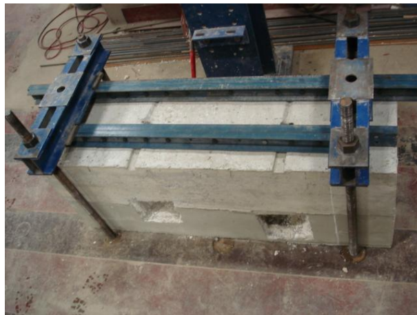
Beams supporting base block
