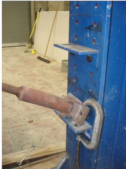
Pin connection at the end of the out-of-plane bracing
