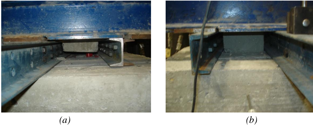
Figure 2.34: Deformation at gap opening of \sim 30.0 , measured at the outermost stiffener on the tension side (a) Gap opening at the tension side toe (b) contact between panel and base block at the compression side toe
