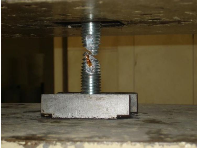
Failure of 3/4" threaded anchor bolt anchor bolt under direct tension (notice necking and elongation in the bar)
