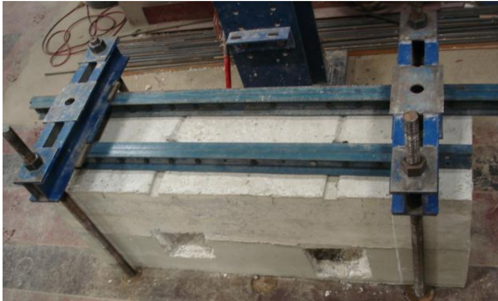
Figure 2.8: Test set-up (concrete base block)
